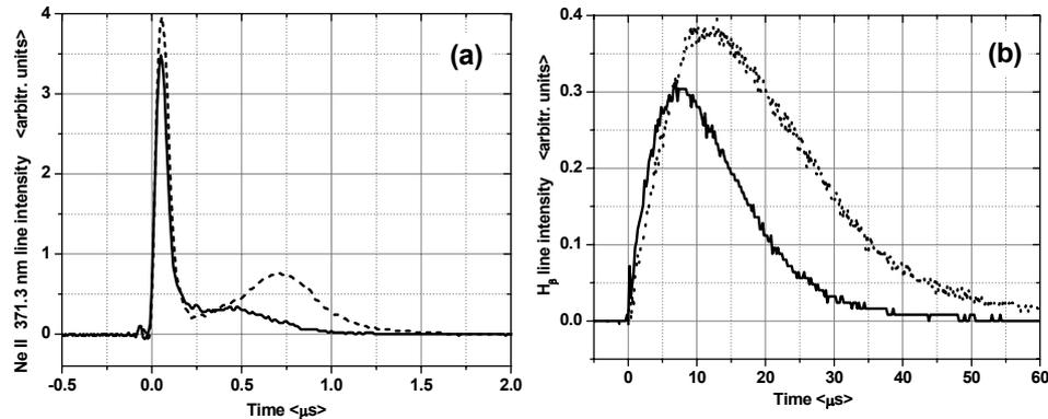
Fig. 13 – Temporal evolution of 3713 Å Ne II line (a) and H<sub>β</sub> line (b), for hydrogen partial pressures:  $7 \times 10^{-2}$  Torr – dashed line, respectively  $1.2 \times 10^{-1}$  Torr – solid line.
