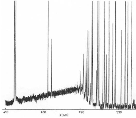
Fig. 7 – Emission spectrum of the cesium afterglow plasma in the range 410–550 nm recorded with an electronic gate of 8  $\mu\text{s}$  widths, opened at 10  $\mu\text{s}$  after the end of the voltage pulse.
