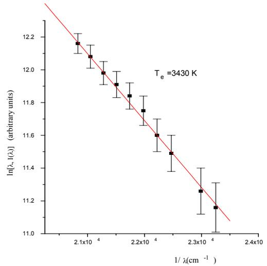
Fig. 8 – Experimental graph  $\ln[\lambda I(\lambda)] = f(1/\lambda)$  and the fitting line.
