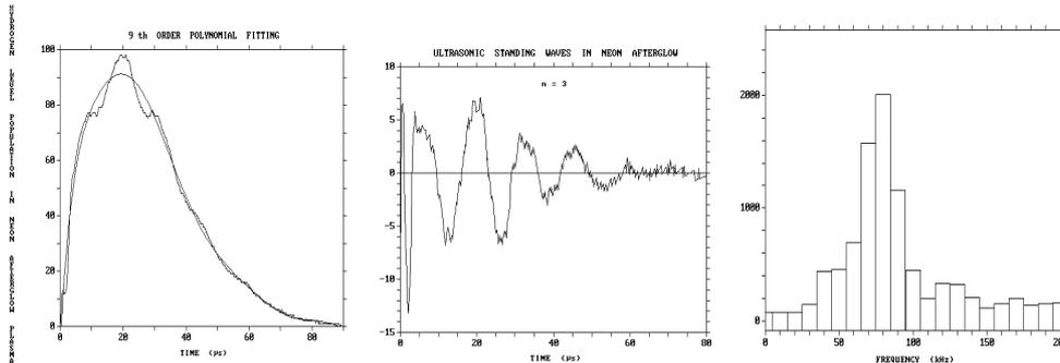
Fig. 5 – The fitted light signal by a 9<sup>th</sup> order polynomial (a); the obtained clean oscillations (b); the Fourier spectrum of the oscillations (c).
