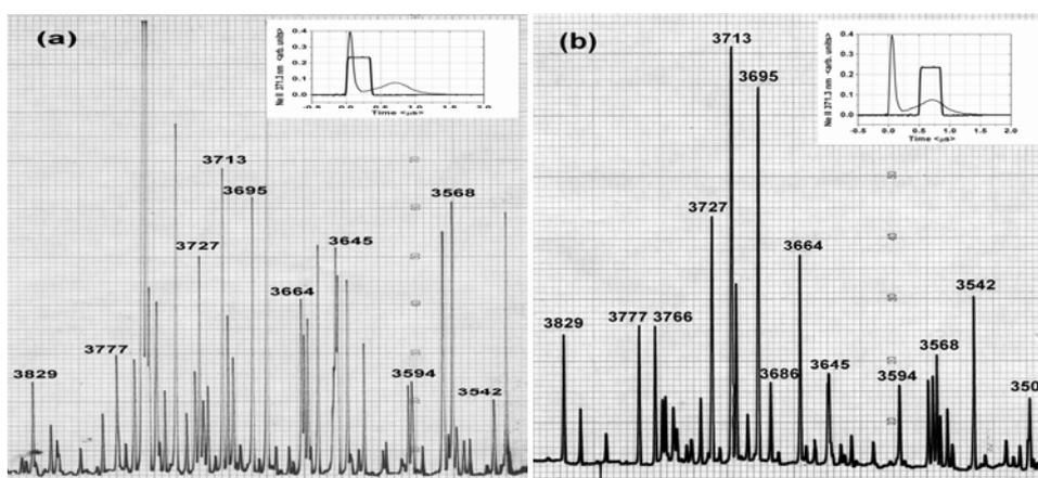
Fig. 3 – The Neon spectra recorded during: a) the current pulse; b) during the afterglow.
