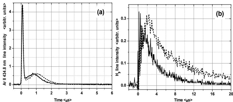
Fig. 14 – Temporal evolution of 4348 Å Ar II line (a) and H<sub>β</sub> line (b), for hydrogen partial pressures:  $7 \times 10^{-2}$  torr – dashed line, respective  $1.2 \times 10^{-1}$  torr – solid line.
