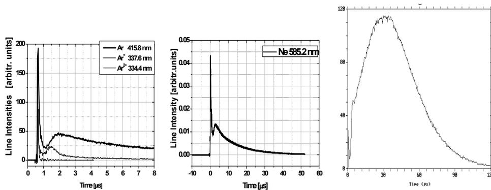
Fig. 2 – The temporal evolution of the light emission of Ar, at 415.8 nm,  $\text{Ar}^+$  337.6 nm,  $\text{Ar}^{++}$  334.4 nm, Ne at 585.2 nm, and  $H_\beta$ , hydrogen being as impurity in Neon.
