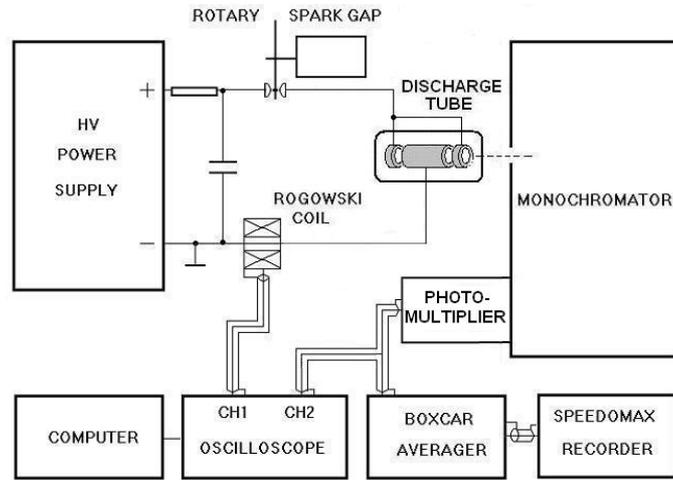
Fig. 1 – Experimental set up with measuring system for temporal resolution spectral analysis.
