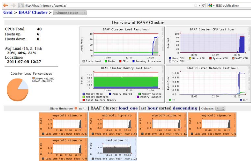
Fig. 2 – Ganglia monitoring web page: the load of the computer cluster during tests.
