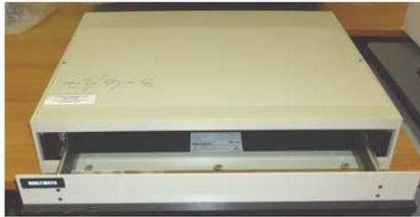
Fig. 1 – The film densitometer – 9721 model (from MULTIDATA System).
