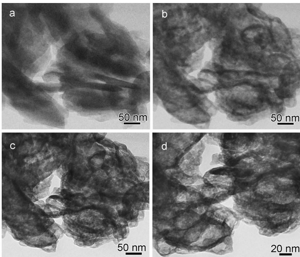
Fig. 3 – Sequence of TEM images corresponding to the ED patterns of Fig. 2, from the same agglomerate of the ZCB specimen exposed to a low current electron beam at  $-160\text{ }^{\circ}\text{C}$ , for different lapses of time: a) 0 min; b) 1 min; c) 5 min; d) 10 min, showing the changes in specimen morphology during the ZCB  $\rightarrow$  ZnO transformation.
