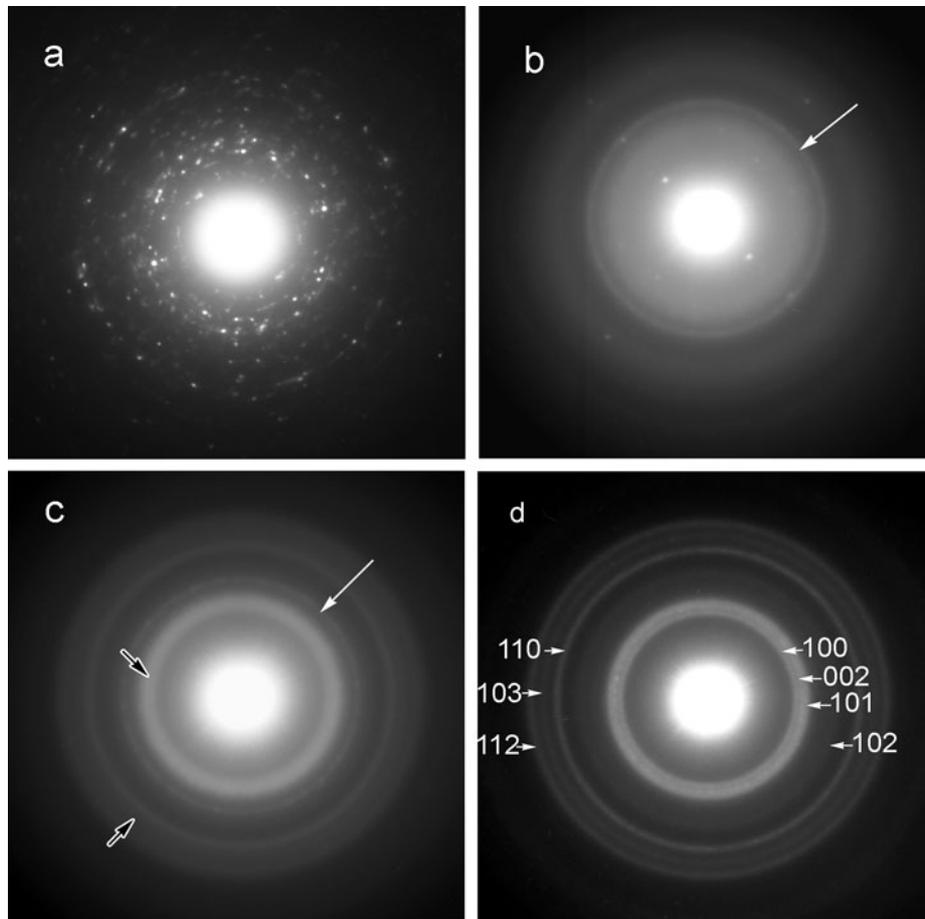
Fig. 2 – Sequence of ED patterns from the same agglomerate of the ZCB specimen exposed to a low current electron beam at  $-160\text{ }^{\circ}\text{C}$ , for different lapses of time, showing the changes in specimen structure during the ZCB  $\rightarrow$  ZnO transformation; white arrow indicates ZCB, black arrows indicate ZnO: a) 0 min, crystalline ZCB; b) 1 min, collapsed lattice of ZCB; c) 5 min, disordered ZnO and traces of ZCB; d) 10 min, indexed ED pattern of nanocrystalline ZnO.
