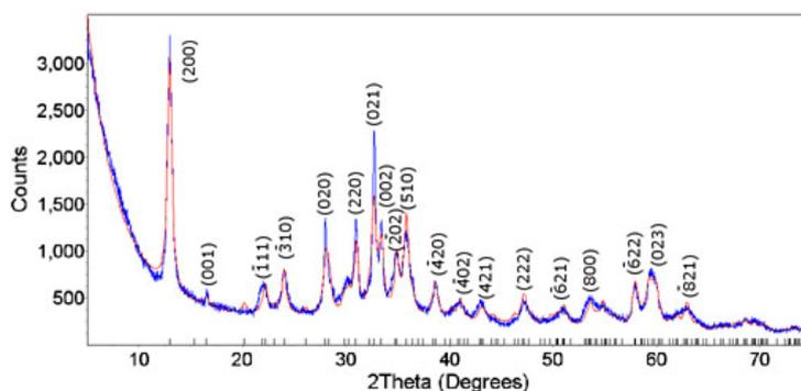
Fig. 1 – The XRD diffractogram of the ZCB and the superposed simulation with parameters from Table 1.
