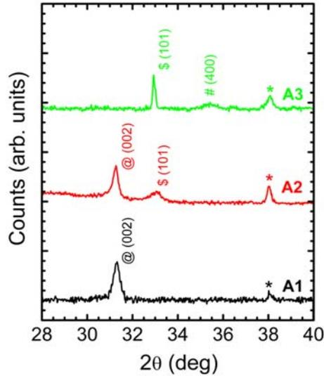
Fig. 3 – XRD curves of the symmetrical  $2\theta/\omega$  scans for samples grown at different substrate temperatures and nitrogen flow rate of 100 sccm (from bottom to top: A1, A2, and A3, respectively). The '@' symbol was assigned to peaks corresponding to InN. Metallic In peaks are highlighted with '\$', whereas  $\text{In}_2\text{O}_3$  is marked with '#'. The diffraction peaks marked with '\*' are a contribution of the sapphire substrate. The spectra are shifted in intensity for clarity.
