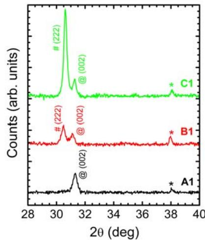
Fig. 1 – XRD curves of the symmetrical  $2\theta/\omega$  scans for samples grown at different nitrogen flow rates and substrate temperature of 550° C (from bottom to top: A1, B1, and C1, respectively). The '@' symbol was assigned to peaks corresponding to InN, whereas In<sub>2</sub>O<sub>3</sub> peaks are marked with '#'. The diffraction peaks marked with '\*' are a contribution of the sapphire substrate. The spectra are shifted in intensity for clarity.
