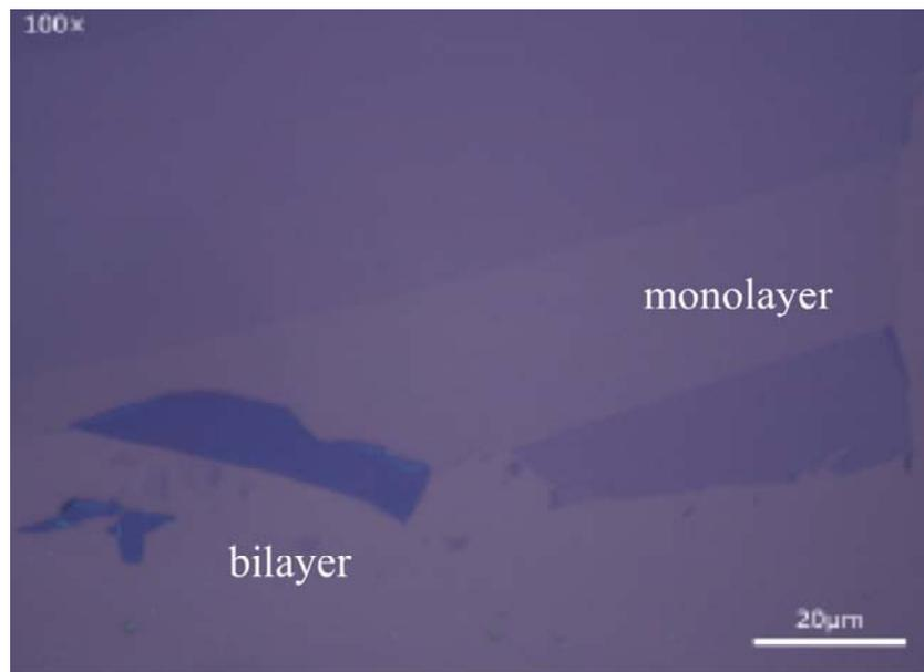
Fig. 3 – Optical picture of graphene bi- and monolayer.
