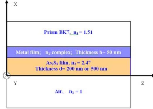
Fig. 2 – The schematic of the plasmonic-waveguide coupling structure.
