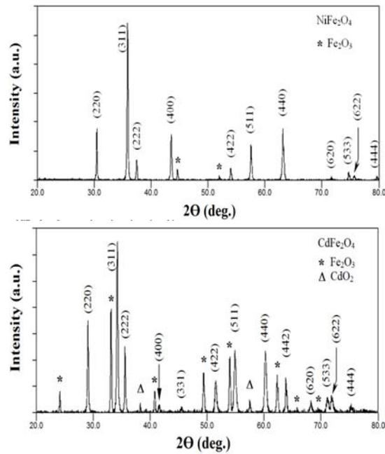
Fig. 2 – XRD patterns for two spinel ferrites ( $\text{NiFe}_2\text{O}_4$  and  $\text{CdFe}_2\text{O}_4$ ).
