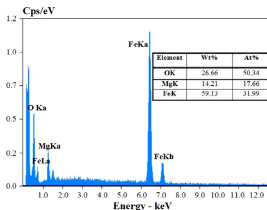
Fig. 5 – EDAX spectrum for  $\text{MgFe}_2\text{O}_4$  ferrite.
