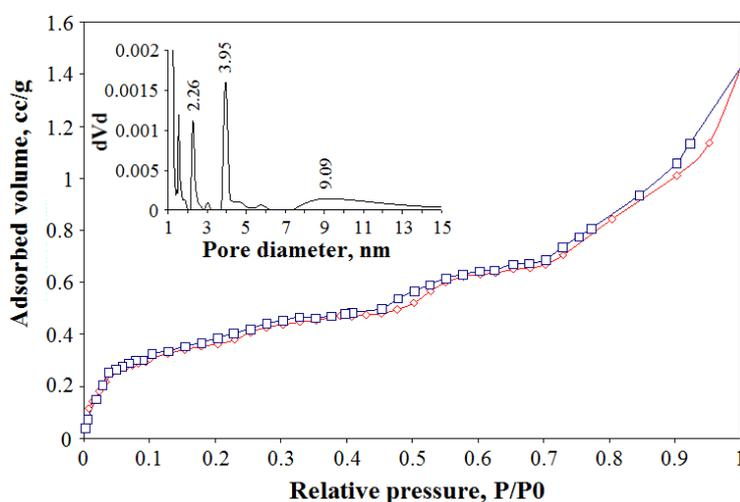
Fig. 4 – Nitrogen adsorption/desorption isotherms at 77K for  $\text{CuFe}_2\text{O}_4$  ferrite powder; symbol romb ( $\diamond$ ) is the adsorption branch and square symbol ( $\square$ ) is the desorption branch. Inset: the pore size distribution graphs.
