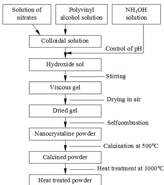
Fig. 1 – Processing of perovskite powders by self-combustion route.
