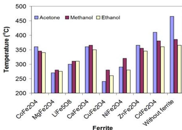
Fig. 6 – Bar diagram, for the minimum combustion temperature of acetone, ethanol and methanol vapor in air in the presence of ferrite catalysts and without catalyst.
