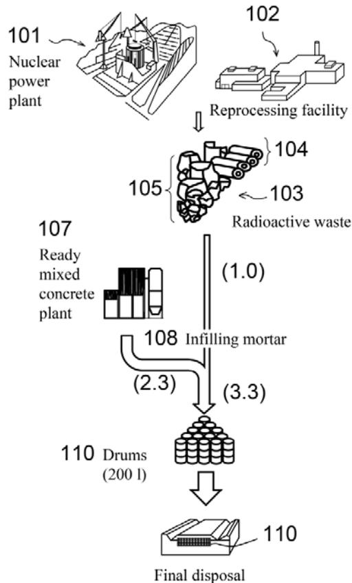
Fig. 1 – Classic method for radioactive concrete processing (referenced from [25]):
