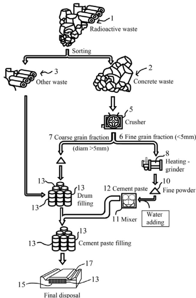
Fig. 4 – Innovative processing method and disposal of radioactive concrete waste referenced from [31]:
