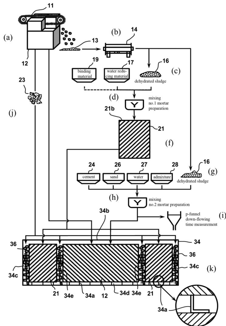
Fig. 3 – Innovative method for radioactive concrete processing (referenced from [28]):
