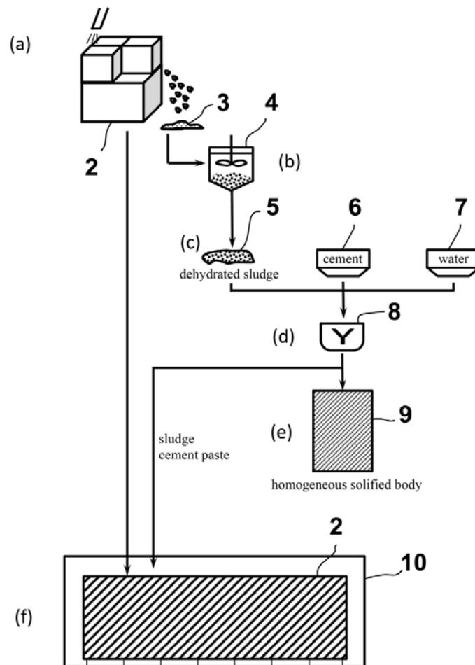
Fig. 2 – Classic method for radioactive concrete processing (referenced from [27]):
