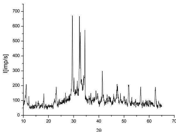
Fig. 5 – The X-ray diffractogram of cement - iron phosphate.
