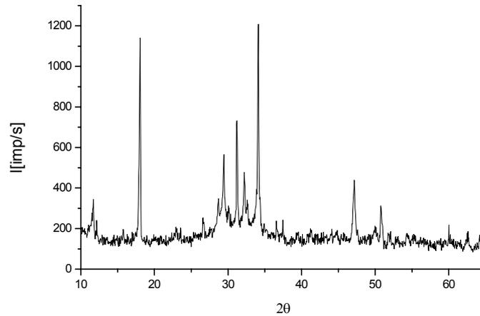
Fig. 1 – The X-ray diffractogram of hydrated cement.
