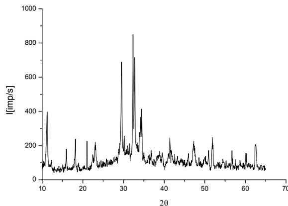
Fig. 4 – The X-ray diffractogram of cement - iron hydroxide.
