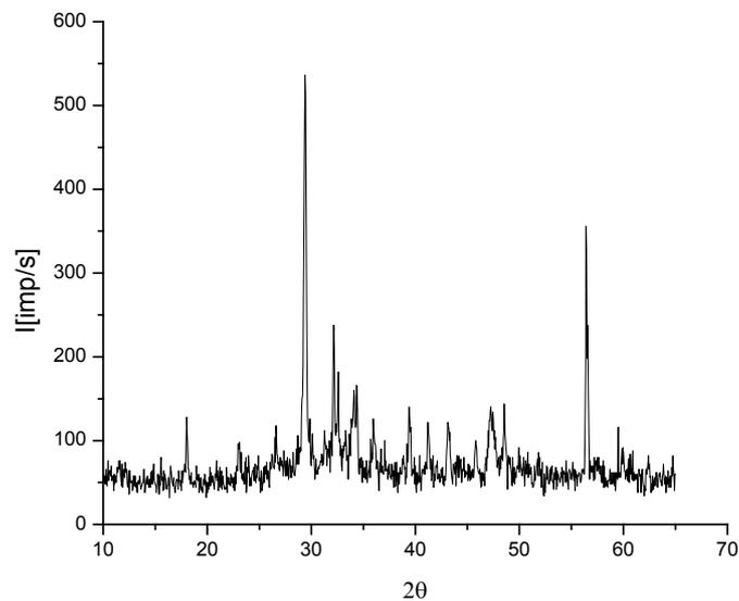
Fig. 2 – The X-ray diffractogram of iron hydroxide.
