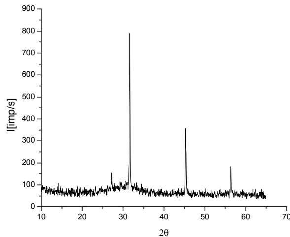
Fig. 3 – The X-ray diffractogram of iron phosphate.
