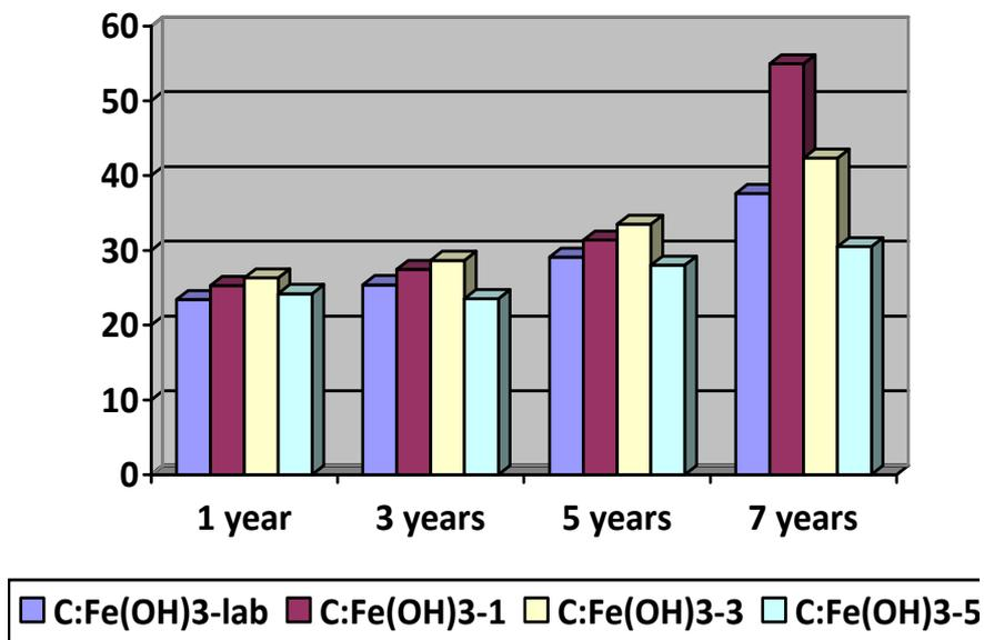
Fig. 2 – Behaviour in time of the compressive strength for cement-iron hydroxide precipitate matrices.
