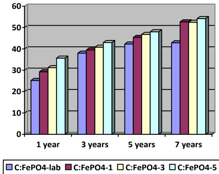
Fig. 3 – Behavior in time of the compressive strength for cement-iron phosphate precipitate matrices.
