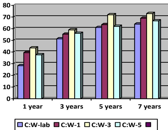
Fig. 1 – Behavior in time of the compressive strength for cement-water matrices.
