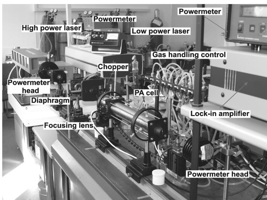
Fig. 1 – A view of the experimental LPAS installation.
