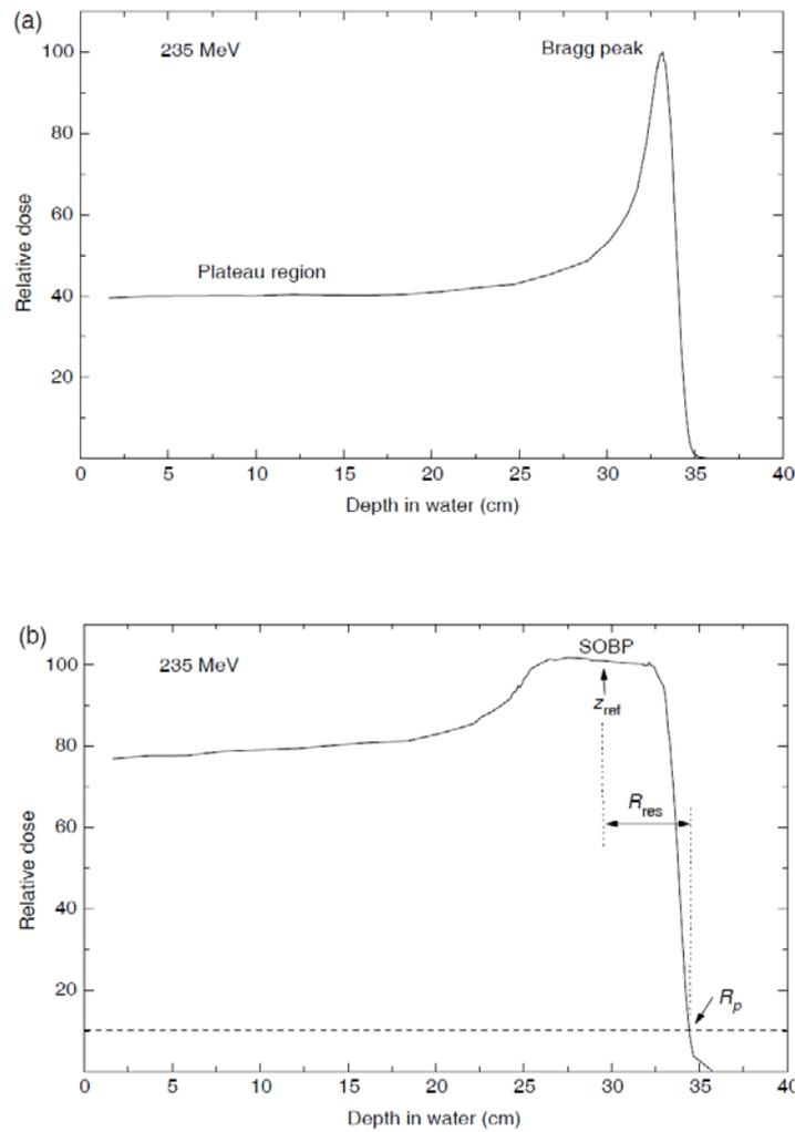
Fig. 2 – Percentage depth dose distributions for a modulated proton beam. There are indicated the reference depth  $z_{ref}$  (middle of the SOBP), the residual range at  $z_{ref}$  used to specify the quality of the beam,  $R_{res}$  and the practical range  $R_p$  [3].
