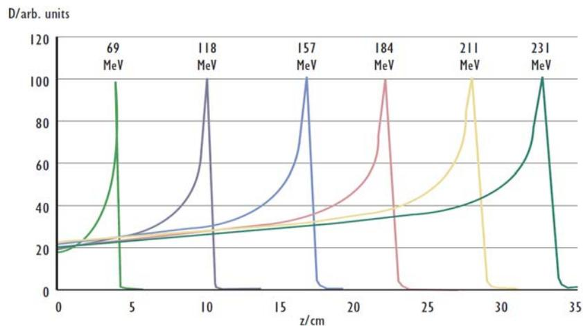
Fig. 1 – Depth in tissue curves as a function of energy for *unmodulated* proton beams [6].
