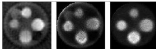
Fig. 6 – The reconstructed images from the non-uniform activity phantom and non-uniform attenuation. From right to left: proposed method, MLEM without attenuation correction, and FBP without attenuation correction method.
