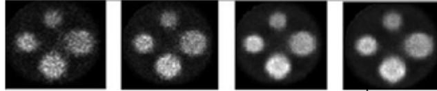
Fig. 10 – The reconstructed images using matrix  $A$  with different activities as input unit: from right to left: activity 300, activity 200, activity 100, and activity 50 million Becquerel.
