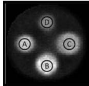
Fig. 3 – Drawing a ROI in different regions of the image to calculate the average pixel values.
