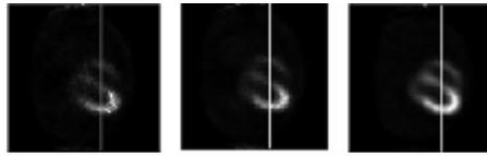
Fig. 8 – From left to right: reference image reconstructed using the proposed method, the reconstructed image using the proposed method, the reconstructed images without attenuation correction.
