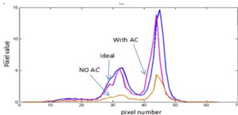
Fig. 9 – The reconstructed image without attenuation correction has less numerical values and contrast than the reference case and the images with attenuation correction during reconstruction.
