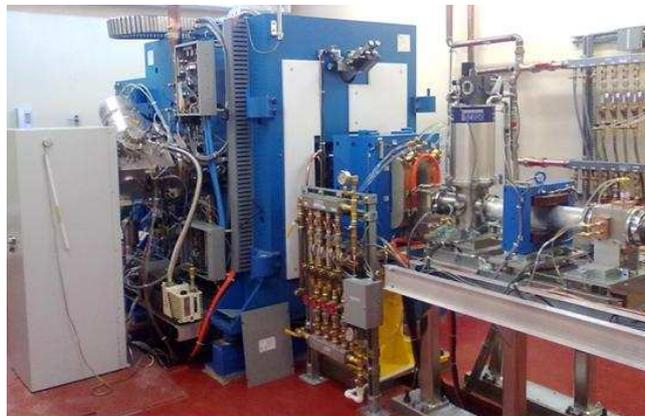
Fig. 9 - TR 19 cyclotron system.
