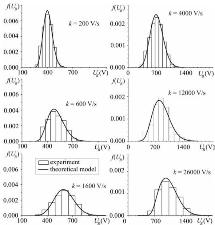
Fig. 3 – Experimental and theoretical breakdown voltage distributions for different increasing voltage rates  $k$  indicated in figure.
