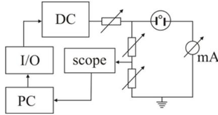
Fig. 1 – Experimental layout.
