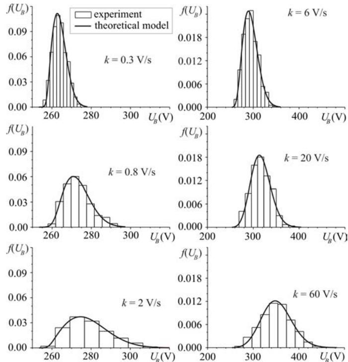
Fig. 2 – Experimental and theoretical breakdown voltage distributions for different increasing voltage rates  $k$  indicated in figure.
