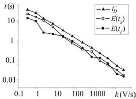
Fig. 4 – Values of  $\bar{t}_D$ ,  $E(t_S)$  and  $E(t_F)$  in function of the voltage increasing rate  $k$ , obtained by theoretical model.
