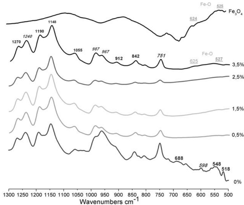
Fig. 4 – FT–IR spectra for PAN/PDLLA composites with different concentration of  $\text{Fe}_3\text{O}_4$ .
