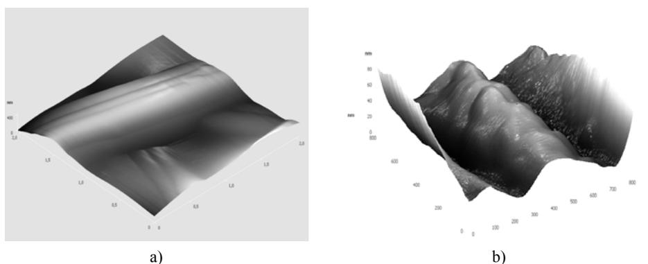
Fig. 3 – AFM images of PAN/PDLLA/  $\text{Fe}_3\text{O}_4$  nanocomposite fibers: a) fibers without magnetical nanoparticles; b) PAN/PDLLA fibers containing 3.5 weight %  $\text{Fe}_3\text{O}_4$  nanoparticles.
