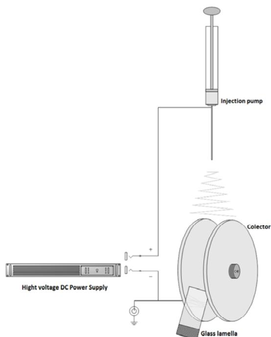
Fig. 1 – Experimental setup for the electrospinning process used to prepare the polymeric magnetic nanofibrous composites.
