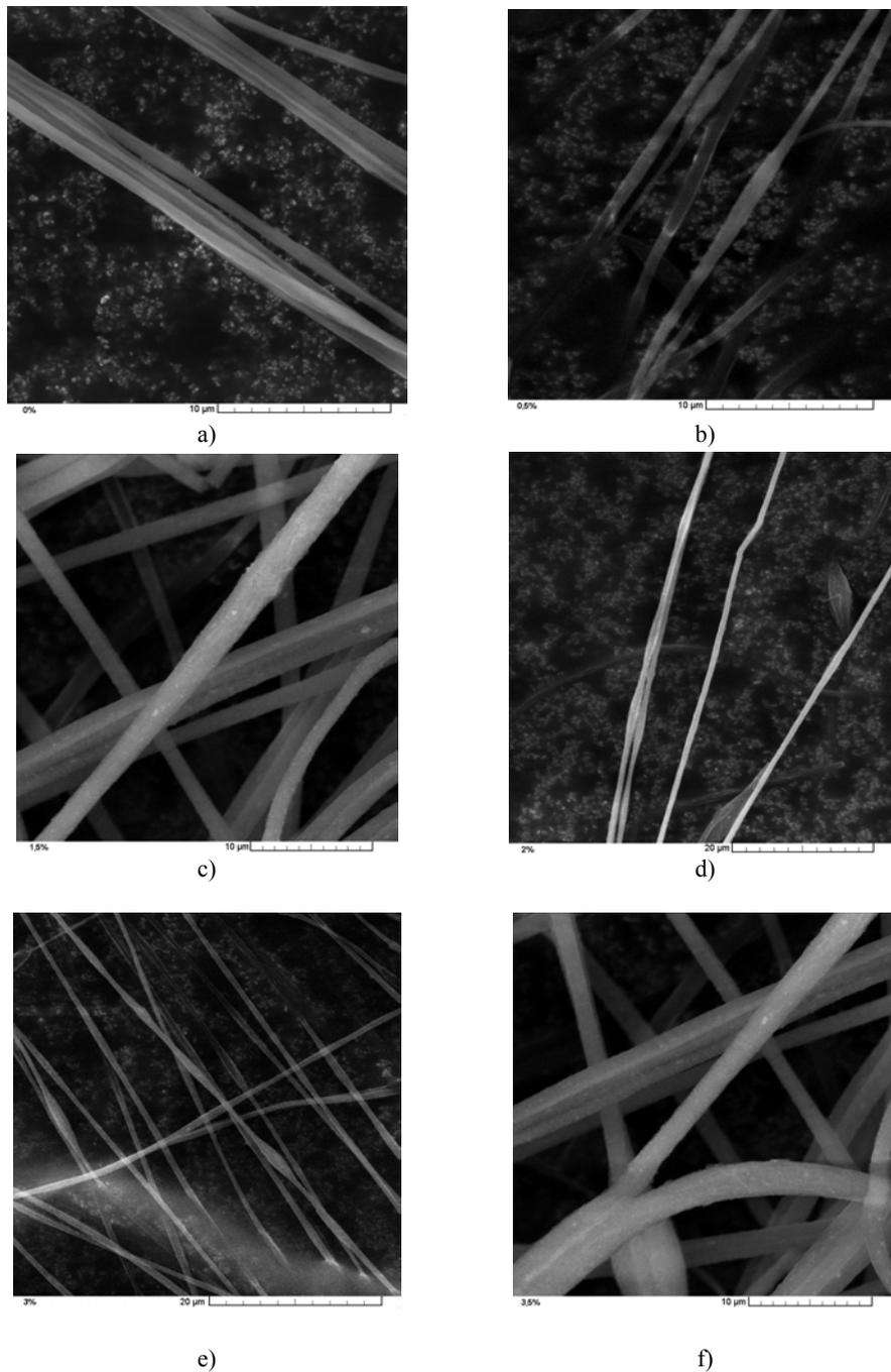
Fig. 2 – Micrographs of PAN/PDLLA- $\text{Fe}_3\text{O}_4$  nanocomposite fibers with different  $\text{Fe}_3\text{O}_4$  nanoparticles weight % content: a) 0%, b) 0,5%, c) 1,5%, d) 2,0%, e) 3,0%, f) 3,5%.
