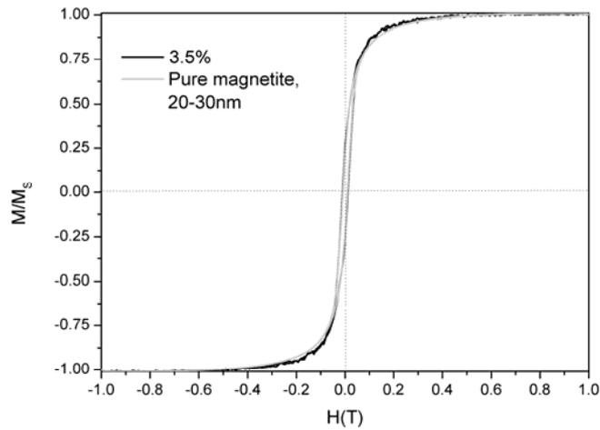
Fig. 6 – Comparison of hysteresis loops for pure magnetite and PAN/PDLLA fibers containing 3.5 % weight  $\text{Fe}_3\text{O}_4$  nanoparticles.
