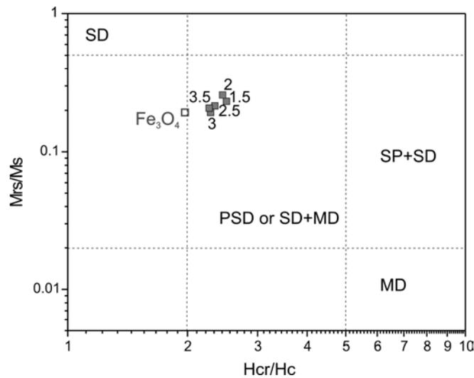
Fig. 5 – Day plot: The ratio of saturation remanence to saturation magnetization,  $M_{rs}/M_s$ , versus ratio of remanence coercivity force to ordinary coercivity force,  $H_{cr}/H_c$ .
