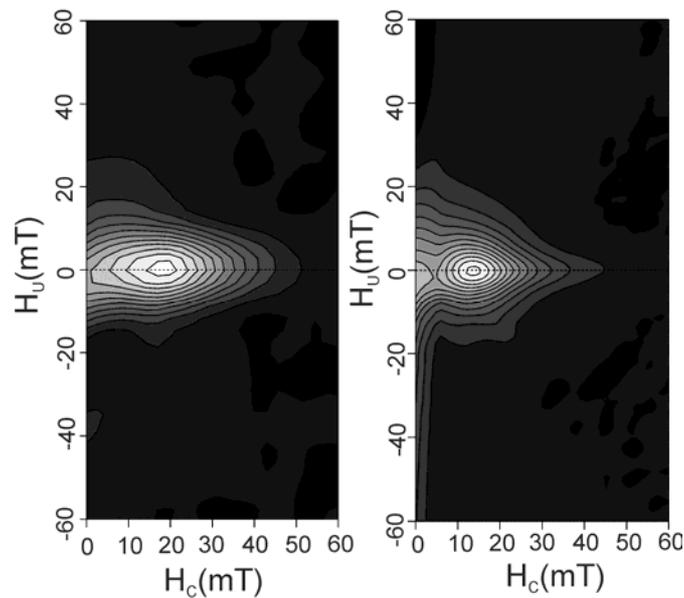
Fig. 7 – First-order reversal curve (FORC) diagrams for PAN/PDLLA fibers containing 3.5 % weight  $\text{Fe}_3\text{O}_4$  nanoparticles (left) and for pure magnetite (right).
