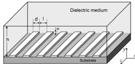
Fig. 2 – Schematic representation of the dielectrophoretic patterning chamber with interdigitated bar electrodes at bottom surface used for DEP nanoparticles separation.
