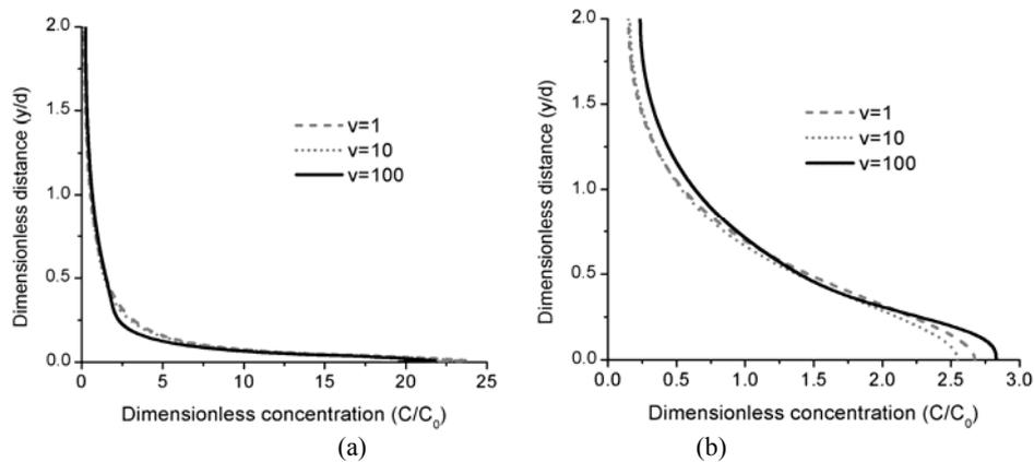
Fig. 7 – Calculated concentration profiles for positive DEP at: a)  $x/d = 0.5$ ; b)  $x/d = 1.0$ . The dimensionless coordinates  $x/d = 0.5$  and  $x/d = 1$  respectively, correspond to the margin of the left electrode and the middle of the distance between electrodes, respectively.
