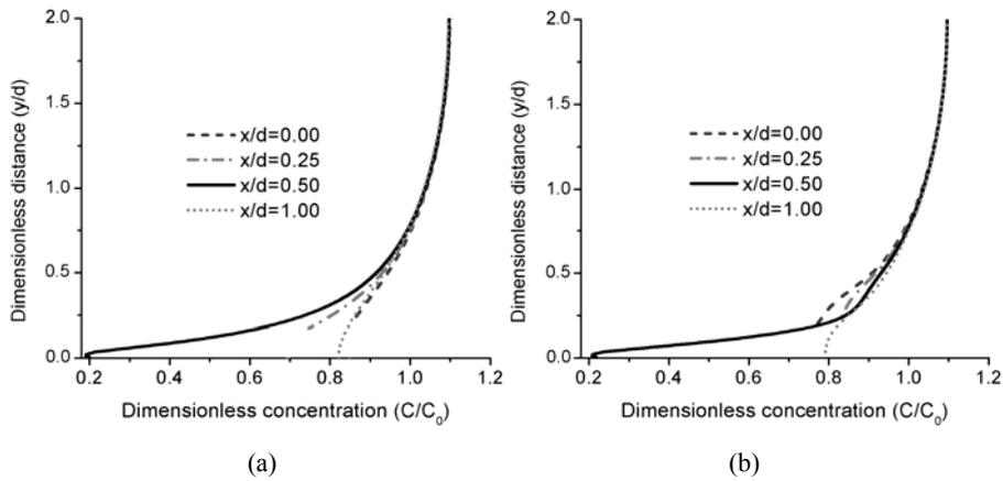
Fig. 8 – Calculated concentration profiles for negative DEP at: a)  $\nu = 1$ ; b)  $\nu = 100$ . The dimensionless coordinates  $x/d = 0$ ,  $x/d = 0.25$ ,  $x/d = 0.5$  and  $x/d = 1$  respectively, correspond to the left margin of the computational domain, the middle of the left electrode, the margin of the left electrode and the middle of the distance between electrodes, respectively.
