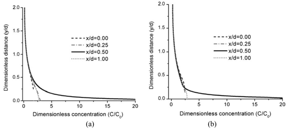
Fig. 6 – Calculated concentration profiles for positive DEP at: a)  $v = 1$ ; b)  $v = 100$ . The dimensionless coordinates  $x/d = 0$ ,  $x/d = 0.25$ ,  $x/d = 0.5$  and  $x/d = 1$  respectively, correspond to the left margin of the computational domain, the middle of the left electrode, the margin of the left electrode and the middle of the distance between electrodes, respectively.
