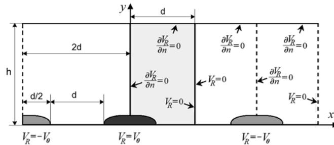
Fig. 3 – The geometry of the computational domain and the boundary conditions for the real part  $V_R$  of the electric potential. The solid lines indicate the basic unit cell.
