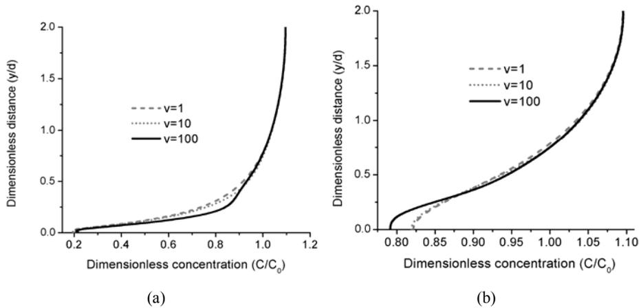
Fig. 9 – Calculated concentration profiles for negative DEP at: a)  $x/d = 0.5$ ; b)  $x/d = 1$ . The dimensionless coordinates  $x/d = 0.5$  and  $x/d = 1$  respectively, correspond to the margin of the left electrode and the middle of the distance between electrodes, respectively.
