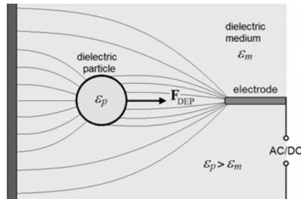
Fig. 1 – Electrically neutral particle in the presence of a spatially non-uniform electric field. The dipole moment induced within the particle results in a translational force and the dielectric spherical particle undergoes a DEP motion.
