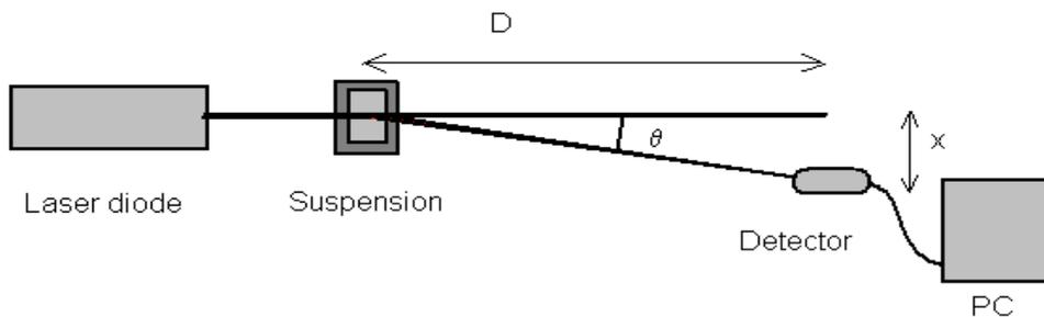
Fig. 1 – The DLS experimental setup, view from above.
