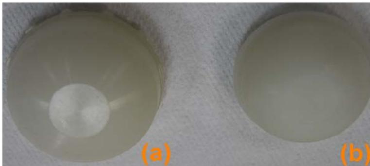
Fig. 3 – Photos of: a) bare; b) BG61 coated UHMWPE acetabular cup.
