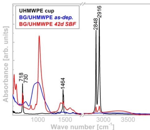
Fig. 1 – FTIR spectra of UHMWPE substrate (black line) and BG61 coatings prior (blue line) and after (red line) 42 days of immersion in SBF.
