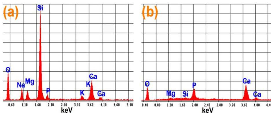
Fig. 5 – EDS spectra of BG61 coatings: a) as-deposited; b) after 42 days of immersion in SBF.
