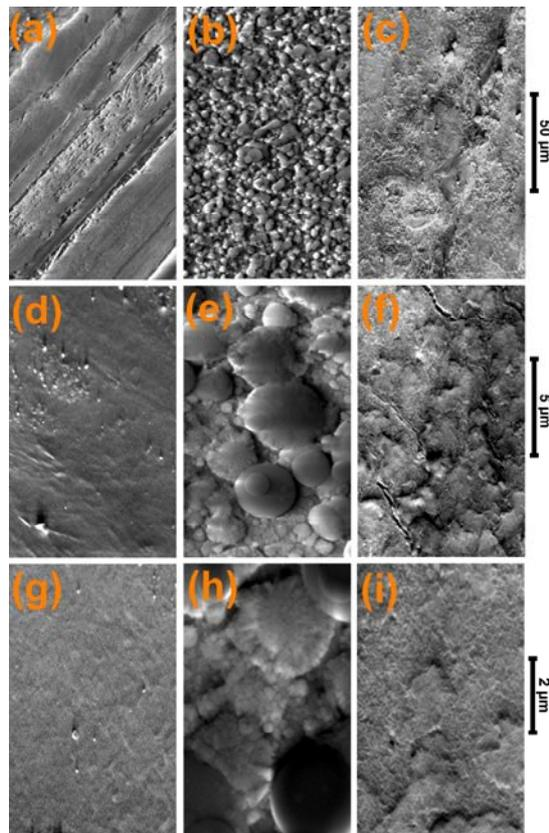
Fig. 4 – SEM micrographs of the UHMWPE acetabular cups: (a, d, g) bare; (b, e, h) biofunctionalized with BG61 films; (c, f, i) after 42 days of immersion in SBF.
