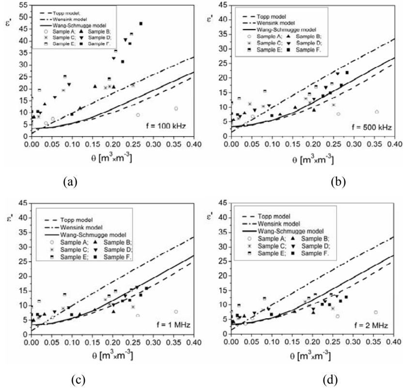
Fig. 2 – A comparison between the theoretical dependence  $\epsilon'(\theta)$ , computed using the Topp, Wensink and Wang-Schmugge models and the experimental dependence  $\epsilon'(\theta)$ , for soil samples at frequencies of: a) 100 kHz; b) 500 kHz; c) 1 MHz; d) 2 MHz.
