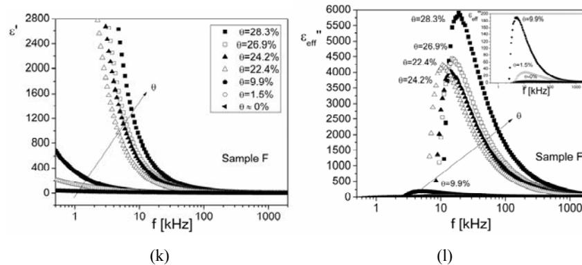
Fig. 1 – The frequency dependence of the real and imaginary components of the complex dielectric permittivity for the investigated soil samples, for the different values of the volumetric water content
