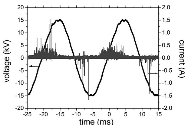
Fig. 2 – Typical waveforms of the discharge voltage and discharge current.
