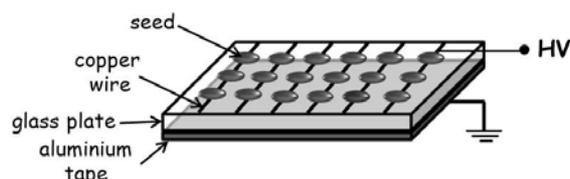
Fig. 1 – Discharge reactor.
