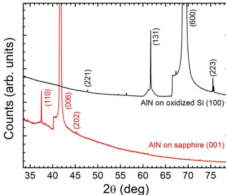
Fig. 2 – XRD spectra of the samples obtained at a laser fluence of  $8 \text{ J/cm}^2$ , on (**top**) amorphous natively oxidized Si (100) and (**bottom**) *c*-cut sapphire substrates, respectively. The spectra are shifted with respect to each other for clarity.
