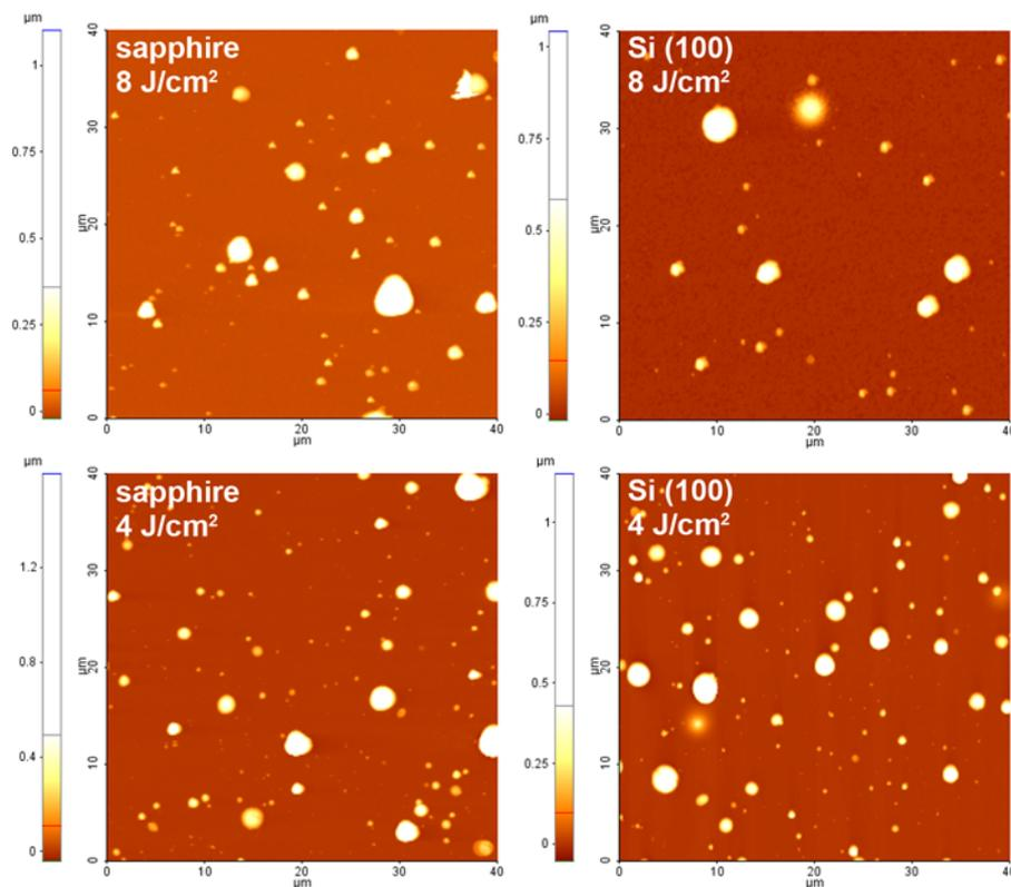
Fig. 3 – AFM micrographs over  $40 \times 40 \mu\text{m}$  areas of AlN thin films grown on *c*-cut sapphire (**left**) and amorphous natively oxidized Si (100) substrates (**right**) at fluences of  $8 \text{ J/cm}^2$  (**top**) and  $4 \text{ J/cm}^2$  (**bottom**), respectively.
