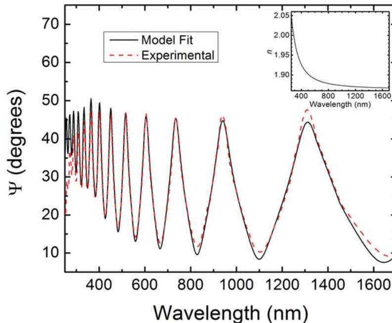
Fig. 1 – Spectral ellipsometry measurement (dashed line) and theoretical fit (continuous line) of the amplitude component ( $\psi$ ) for an AlN thin grown on amorphous natively oxidized Si (100) substrate, using a laser fluence of  $8 \text{ J/cm}^2$ . The inset shows the wavelength dependence of the refractive index used in our model.
