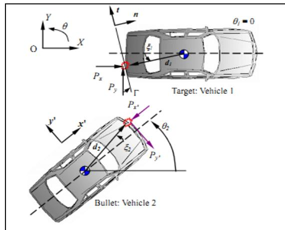
Fig. 2 – The collision scenario [29]. The colored versions could be accessed at <http://www.infim.ro/rfp/>.
