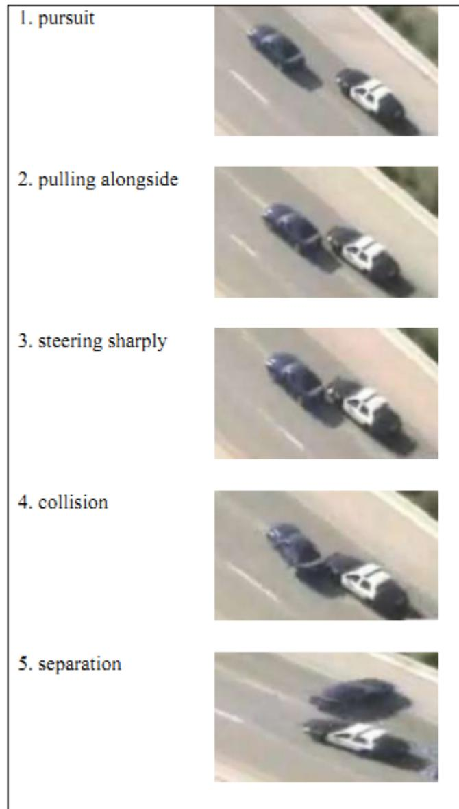
Fig. 3 – The states of PIT maneuver [30, 32]. The colored versions could be accessed at <http://www.infim.ro/rp/>.
