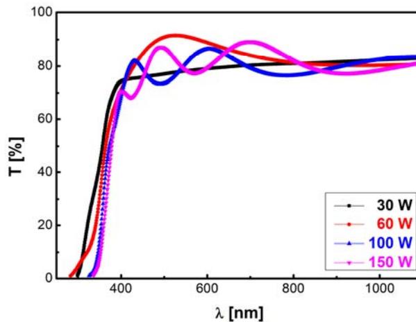
Fig. 2 – Transmission spectra for the AZO films sputtered at different cathode powers.
