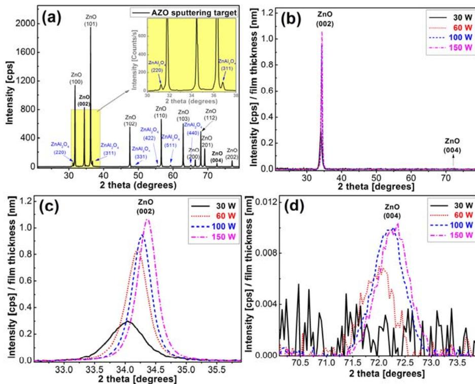
Fig. 1 – Comparative X-ray diffraction patterns for: a) AZO target; b) AZO sputtered films; c) 002 peak region detail; d) 004 peak region detail for the AZO films.
