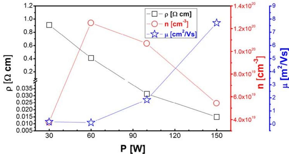
Fig. 4 – The AZO films' electrical resistivity ( $\rho$ ), mobility ( $\mu$ ) and carrier concentration ( $n$ ) function of the sputtering power.
