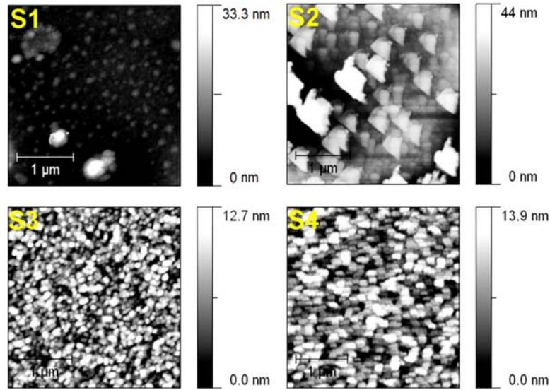
Fig. 3 – Morphology dependence of AZO films on sputtering power, as revealed by the AFM analyses.
