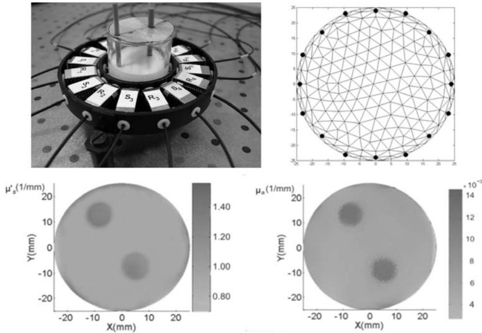
Fig. 6 – The liquid phantom with 1% Lipofundin and two glass tubes filled with hemoglobin.
