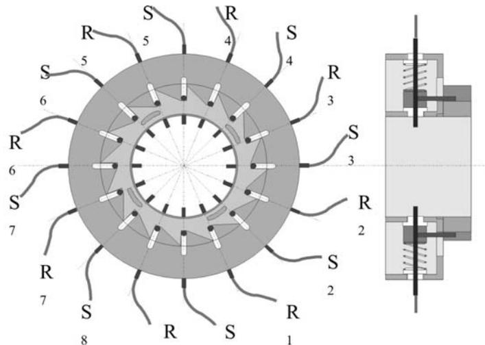
Fig. 4 – The optode and the radial distribution of the fiber bundle.
