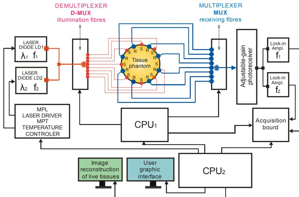
Fig. 3 – An overview of the DOT experimental setup.
