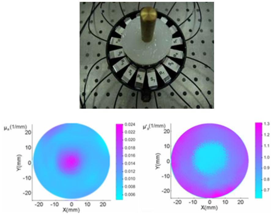
Fig. 7 – The rubber phantom with a central opaque metal bar.
