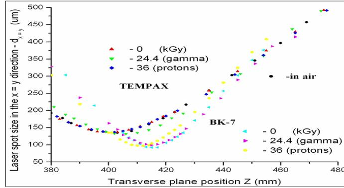
Fig. 7 – The beam diameter variation depending on the position of the plane perpendicular to the direction of propagation –  $Z$  for our four situations in which the samples were measured (air, non-irradiated, 24.4 kGy gamma irradiated and, respectively, 36 kGy protons irradiated).
