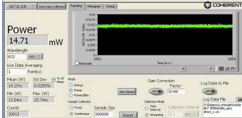
Fig. 5 – Example of measuring the maximum power transmitted through the air and its stability during 35 minutes.
