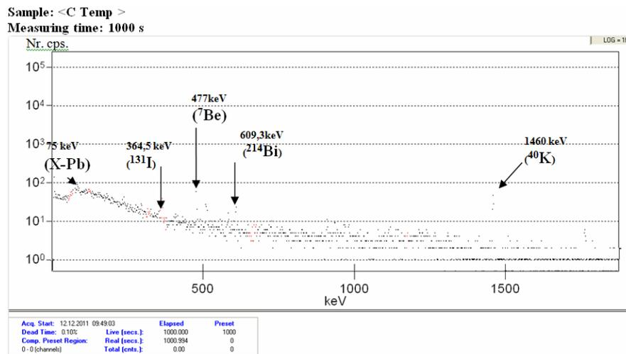
Fig. 3 – Gamma spectra of TEMPAX irradiated samples.
