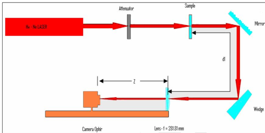
Fig. 6 – The experimental setup used to measure the spatial parameters of the laser beam after passing through the irradiated samples.
