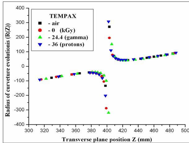
Fig. 8a – Illustration of the measured radius of curvature evolution of the artificial laser beam (stigmatic) in air, to blank glasses, to the 24.4 kGy gamma dose, and to the 36 kGy dose of protons as a function of propagation distance  $-Z$  for TEMPAX glass.
