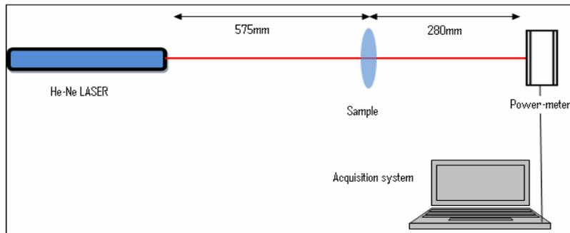
Fig. 4 – A schematic diagram of the measuring system of the power transmitted through the samples.
