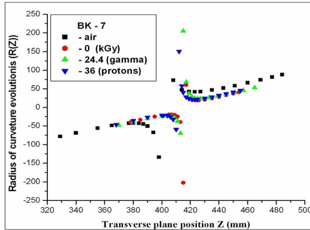
Fig. 8b – Illustration of the measured radius of curvature evolution of the artificial laser beam (stigmatic) in air, to blank glasses, to the 24.4 kGy gamma dose, and to the 36 kGy dose of protons as a function of propagation distance  $-Z$  for BK-7 glass.
