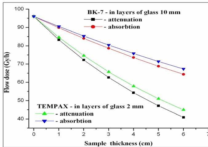
Fig.1 – The dose flow as a function of sample thickness.
