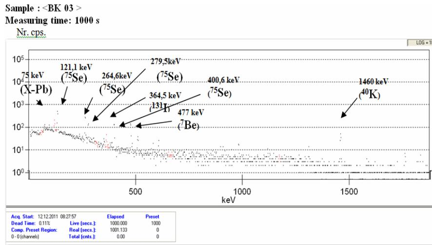
Fig. 2 – Gamma spectra of BK-7 irradiated samples.
