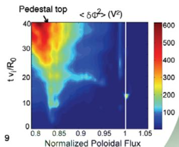
Fig. 4.1 – ITG non-linear simulation using a global/full-f GK from [14] showing the fluctuation pattern evolving in time as a function of the radial position. The white line corresponds to the position of the separatrix.
