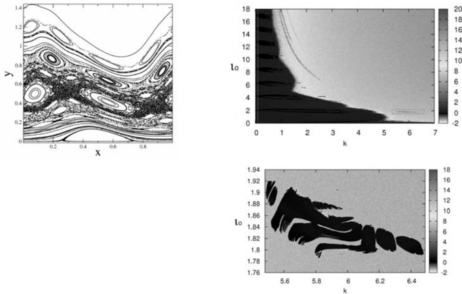
Fig. 2.1 – Phase space portrait of the Tokamak in the case of a strong perturbation (a – left), and Lyapounov exponents calculated for various safety factor values on the magnetic axis and various values of the perturbation amplitude (b – right top). In c are (right bottom) showing the details of the Lyapounov exponents corresponding to the small green area of b. Lowest values of the Lyapounov exponents are in the blue-black colors. Plots are from [7].
