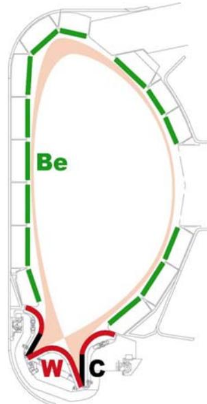
Fig. 1.2 – Geometry of the Tokamak in this case with a single X-point at the bottom of the machine. The divertor is made of tungsten (except for some carbon tiles) as opposed to the wall made of Beryllium in JET Tokamak in the UK and in ITER [2].
