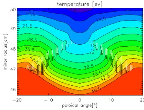
Fig. 2.5 – Plasma temperature near the edge from MHD calculations using Eq. (2) reproduces the two “arms”. The prolongation of these features to the edge (top of the figure) leads zone at higher temperature than the rest of the edge region.
