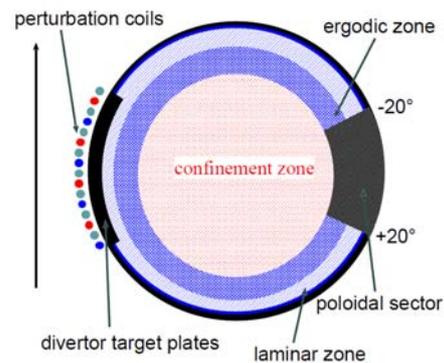
Fig. 2.2 – TEXTOR equipped with sets of resonance magnetic perturbation coils on the inner side of the Tokamak. In this experiment by switching on/off different sets of coils it is possible to induce time periodic perturbations acting on different rational values of the safety factor [8].
