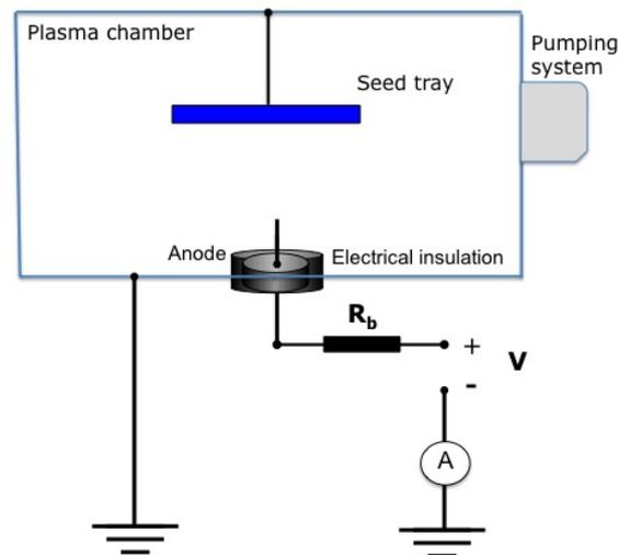
Fig. 1 – Schematic set up of plasma system.
