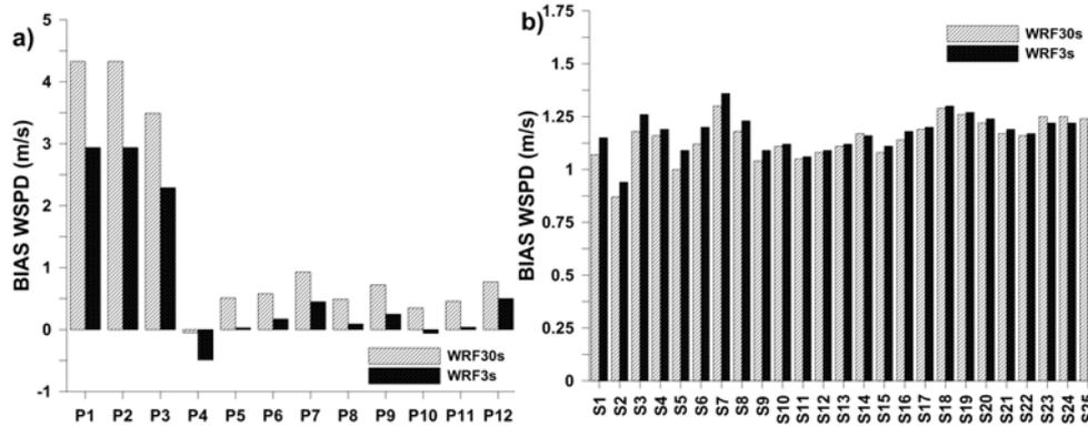
Fig. 4 – Wind speed BIAS for mountain stations (a) and low altitude stations; (b) for 15 January – 15 February 2012 period.
