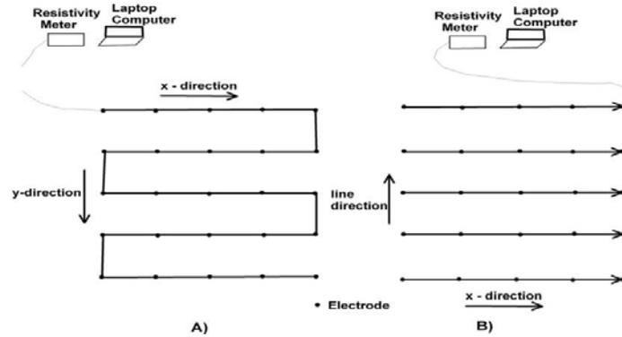
Fig. 1 – A typical arrangement of electrodes for a 3-D survey: A) 3-D survey; B) parallel lines with equal distance.
