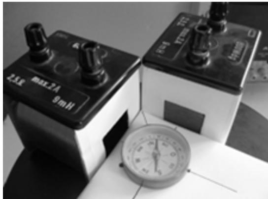
Fig. 5 – Because of the interaction between the ferromagnetic core and compass needle, the needle turns towards R.
