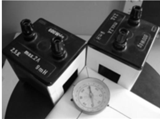
Fig. 4 – The compass needle is aligned with the horizontal component of the Earth's magnetic field.
