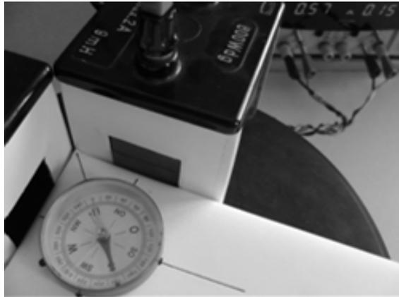
Fig. 9 – The position of the compass needle for  $I_R = 0.15$  A and  $I_L = 0.57$  A.
