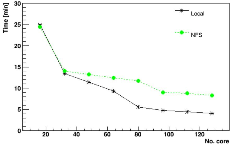
Fig. 4 – Execution time variation as a function of the number of processing cores using ATLAS data.
