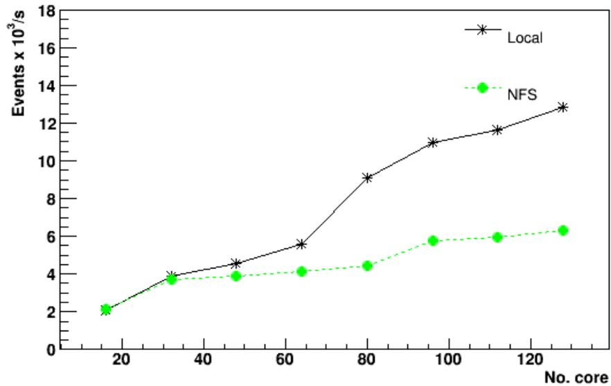
Fig. 5 – Number of events per second as a function of the number of processing cores using ATLAS data.
