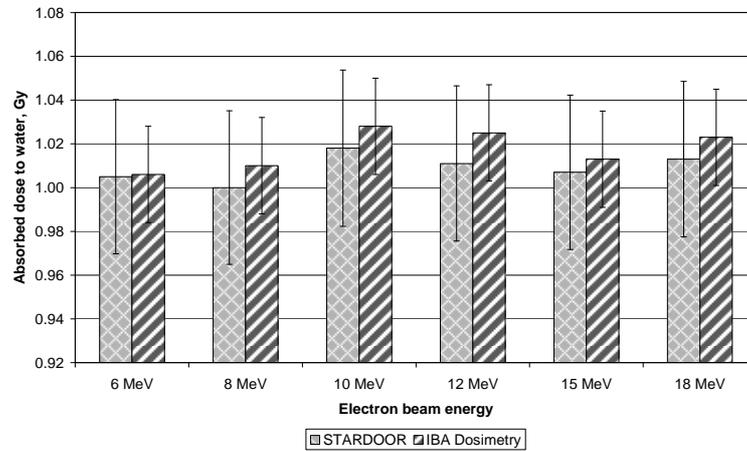
Fig. 1 – Diagram of the measurement results of absorbed dose in water and the expanded uncertainty for the two laboratories.
