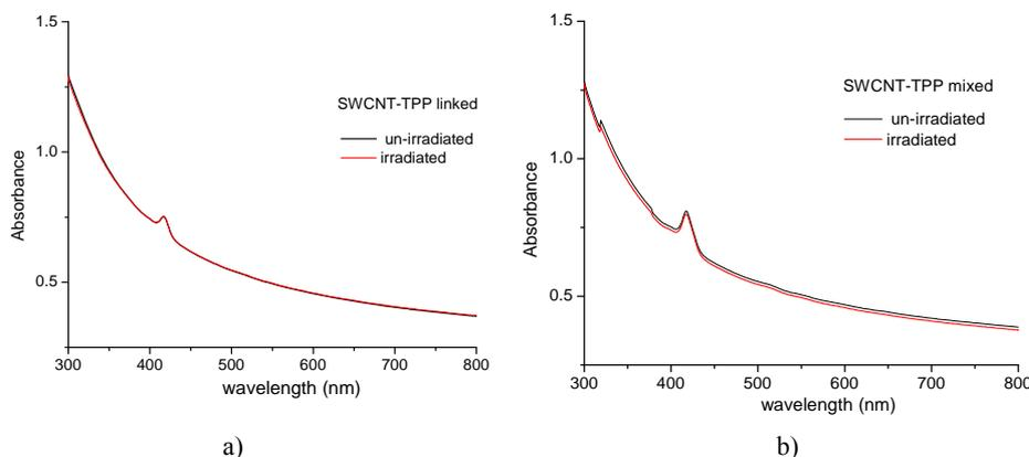
Fig. 4 – The absorption spectra for un-irradiated/irradiated samples: a) SWCNT-TPP linked, b) SWCNT-TPP mixed (online color).
