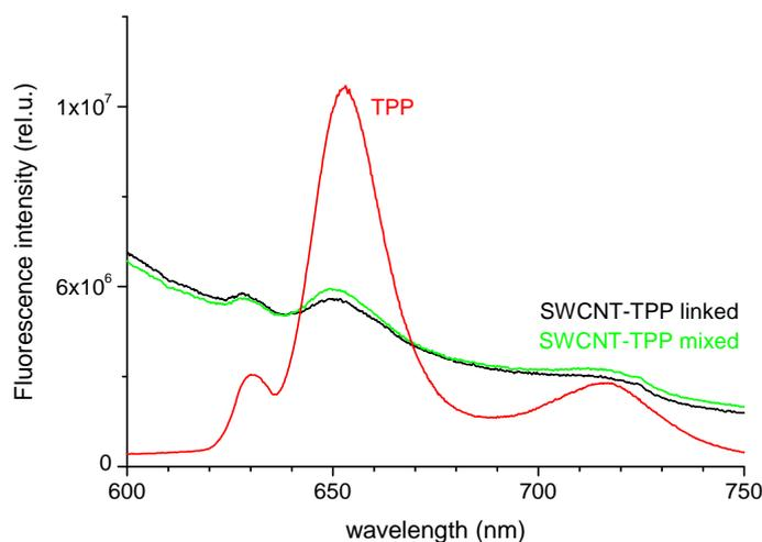
Fig. 6 – The LIF spectra for mixed and linked compounds compared with TPP spectrum (online color).
