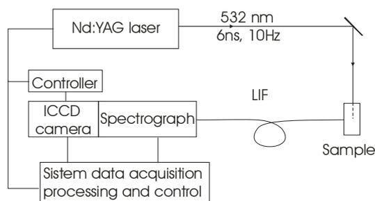
Fig. 2 – The LIF experimental set-up.
