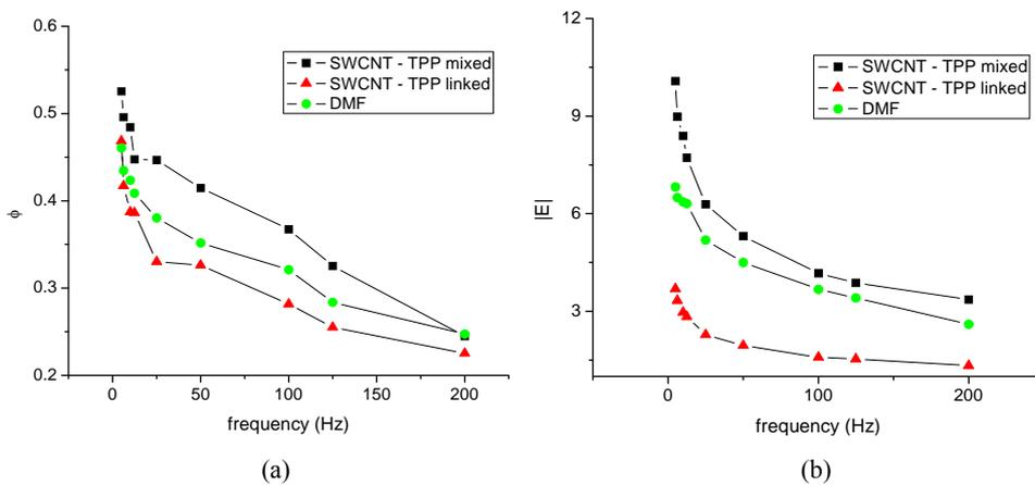
Fig. 5 – Visco-elastic modulus ( $|E|$ ) (a) and the phase lag ( $\Phi$ ) (b) values (online color).
