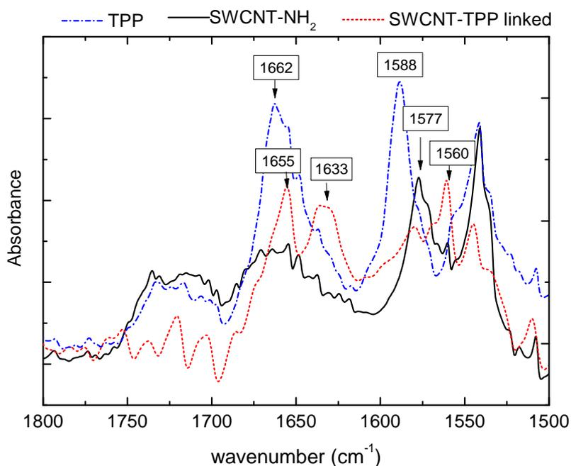
Fig. 7 – The FTIR spectra for TPP, SWCNT-NH<sub>2</sub>, and the conjugated compound (online color).
