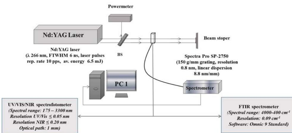
Fig. 3 – Laser exposure experimental set-up and the used survey devices.
