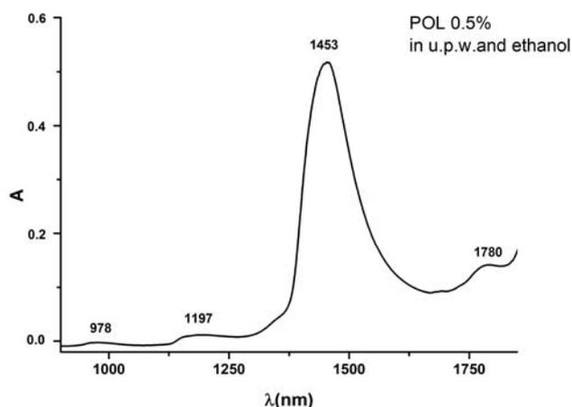
Fig. 5 – The absorption spectrum of POL solution in NIR spectral range.
