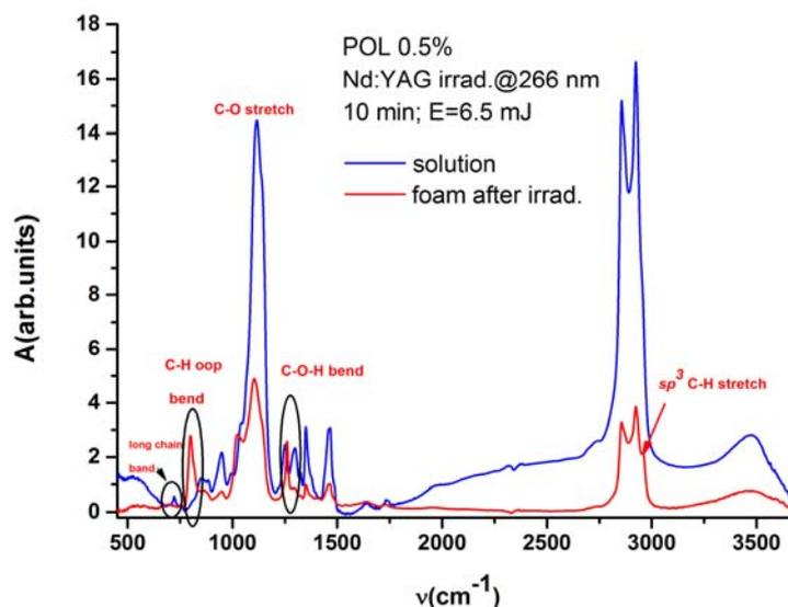
Fig. 7 – FTIR spectra of the 10 min exposed solution to pulsed Nd:YAG laser radiation (on-line color).
