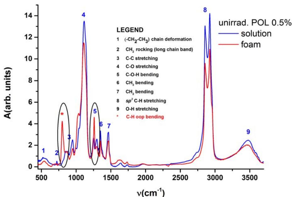
Fig. 6 – FTIR spectra of unirradiated POL (on-line color).
