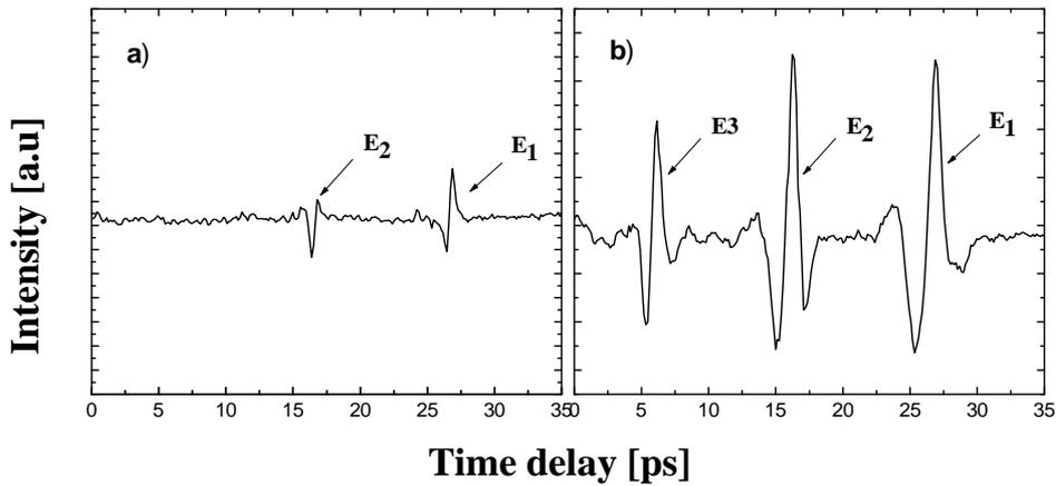
Fig. 4 – Recorded THz waveforms for  $R$  coefficient kept at 40% and different amount of total energy  $E_T$ : a) 1 mJ, b) 5.3 mJ.
