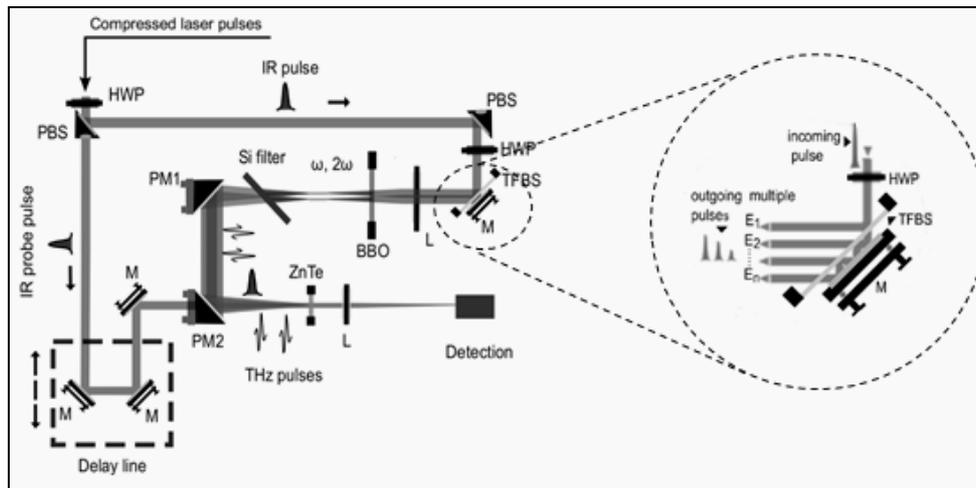
Fig. 3 – Experimental setup for THz emission from multiple filaments. HWP, half-wave plate; PBS, polarizing beam splitter; TFBS, thin film beam splitter; M, 45° high reflectivity dielectric mirrors; L, achromatic lenses; BBO  $\beta$ -barium borate crystal, Si filter, silicon filter PM1, PM2, off-axis 90° gold coated parabolic mirrors; ZnTe, zinc telluride crystal; Detection, Z-Omega auto-balanced detector ABL-100.
