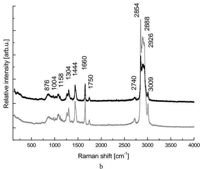
Fig. 3 – a) SERS spectra taken on smears laid on Ag-coated scalpel blades (corresponding respectively to the samples shown in Fig. 2a, b, c; b) SERS spectra of pure fat (black-dog; gray-cat) corresponding to images a and c in Fig. 2.
