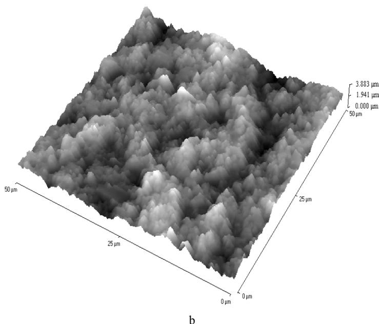
Fig. 1 – AFM measurements performed over a  $50 \mu\text{m}^2$  area on a) raw stainless steel surgical blades (RMS roughness is  $0.11 \mu\text{m}$ ); b) silver coated surgical blades (RMS roughness is  $0.5 \mu\text{m}$ ).
