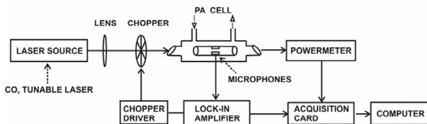
Fig. 1 – Schematic of the CO<sub>2</sub> laser based PA set-up.
