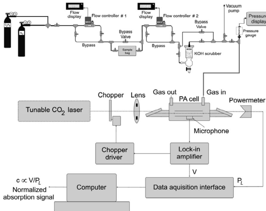
Fig. 1 – Schematic of the CO<sub>2</sub> laser-photoacoustic spectroscopy instrument.
