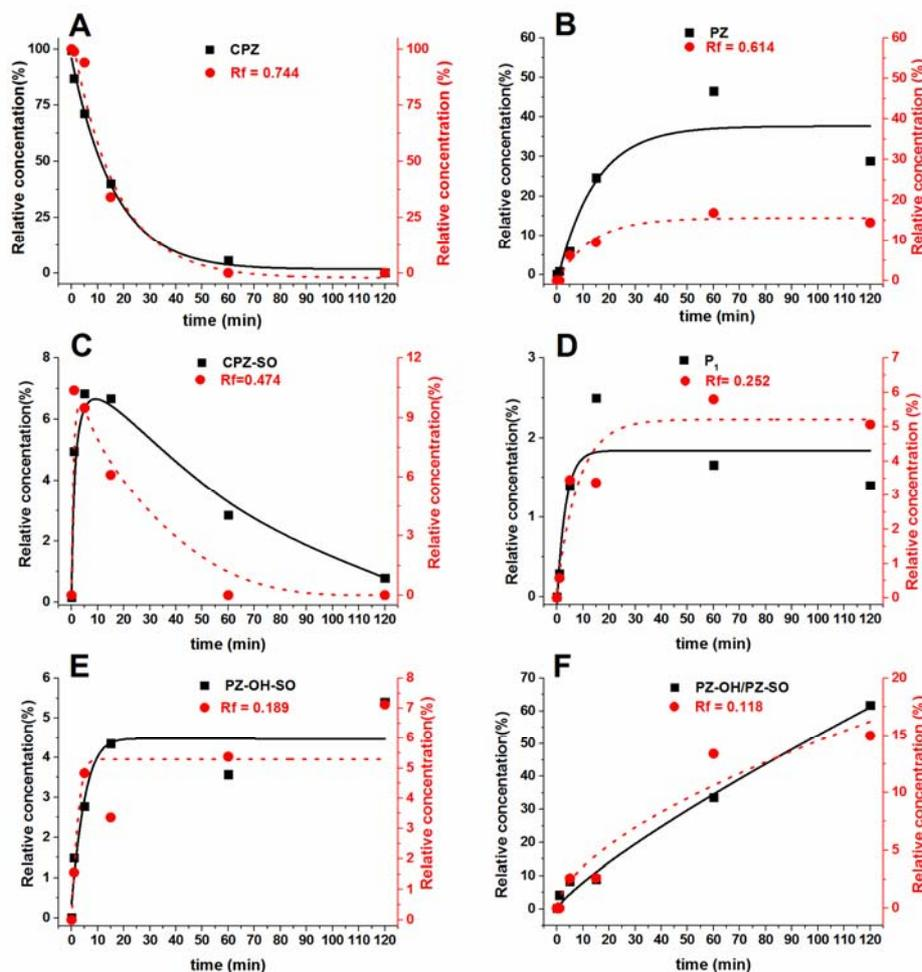
Fig. 3 – The evolution of the relative concentration of the photoproducts identified *via* LC-TOF/MS (continuous line) and *via* JustTLC (dotted line); online color.
