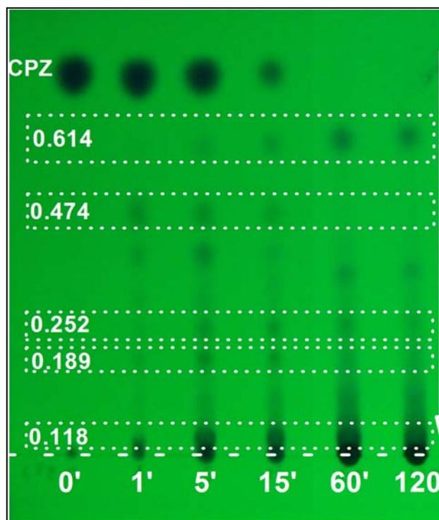
Fig. 2 – TLC plate with unirradiated and irradiated CPZ for 1, 5, 15, 60, and 120 min, visualized at 254 nm (online color).
