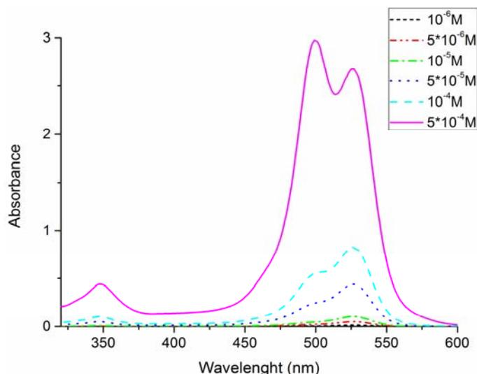
Fig. 4 – The absorption spectra of solutions of different concentrations of Rh6G in ultrapure water.
