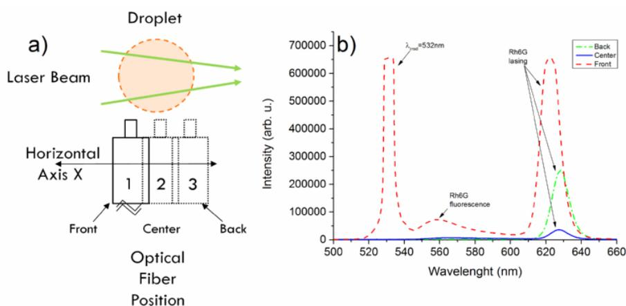
Fig. 6 – a) Cartoon depicting the optical fiber for measuring fluorescence at different positions on a droplet; b) laser induced fluorescence of Rh6G solution measured at different position on the equatorial plan of a droplet.
