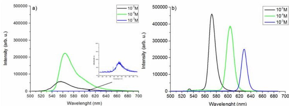
Fig. 5 – Comparison between fluorescence spectra of Rh6G solution emitted by droplet and bulk (spectrophotometric cuvette) at different concentrations.
