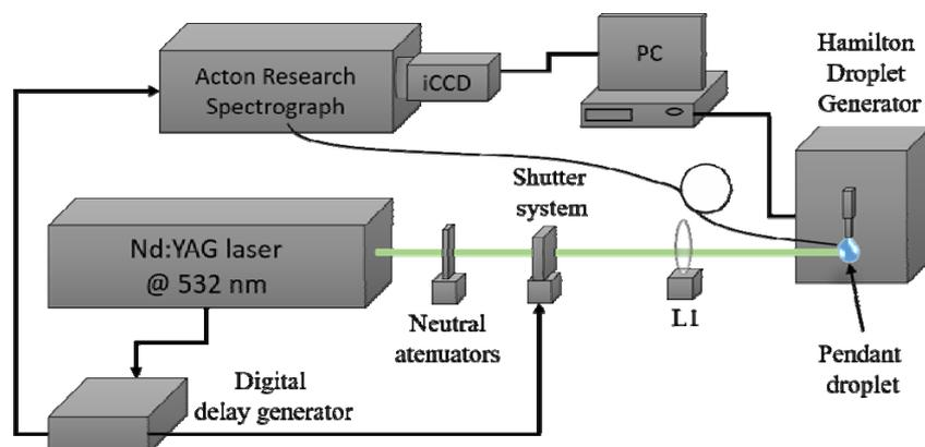
Fig. 1 – Experimental set-up used for irradiation of pendant droplets seeded with solutions of Rh6G. Evolution of the laser beam waist is represented in Fig. 2.
