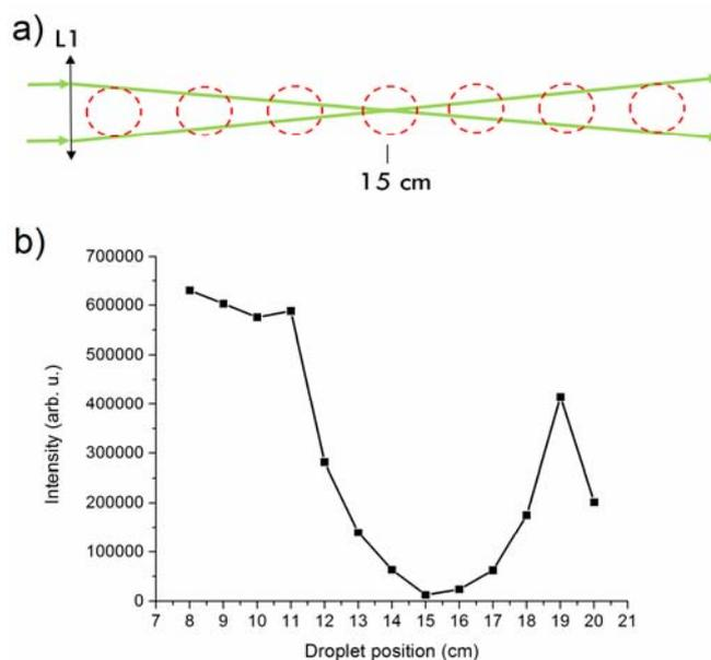
Fig. 2 – a) Cartoon depicting the evolution of the laser beam waist; b) intensity of laser induced fluorescence spectra of Rh6G  $10^{-5}$ M solutions in ultrapure water taken in different focus positions.
