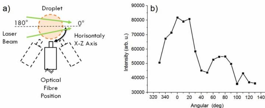
Fig. 7 – a) Cartoon depicting the experimental set-up for measuring fluorescence at different angles on a droplet; b) intensity of the signal measured at different angles.
