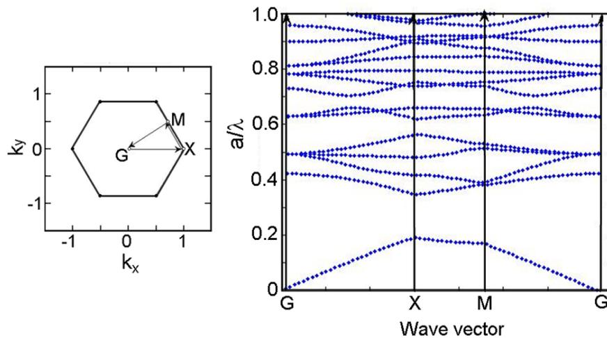
Fig. 2 – Irreducible part of the 1<sup>st</sup> Brillouin zone (left) and the photonic band structure of a triangular lattice for a GaN two-dimensional photonic crystal with  $R = 0.25a$  ( $R$  – radius of holes;  $a$  – lattice constant), calculated for TM modes (right).
