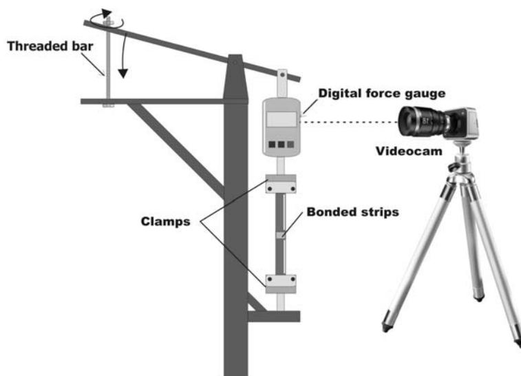
Fig. 2 – Schematics of the bonding strength testing device.
