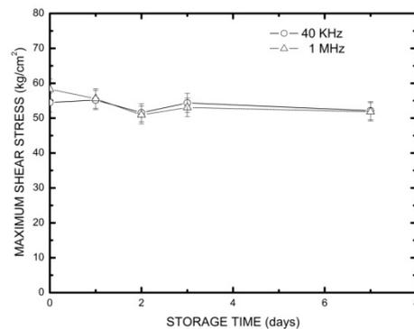
Fig. 5 – Evolution of shear strength after the treatment in plasma.
