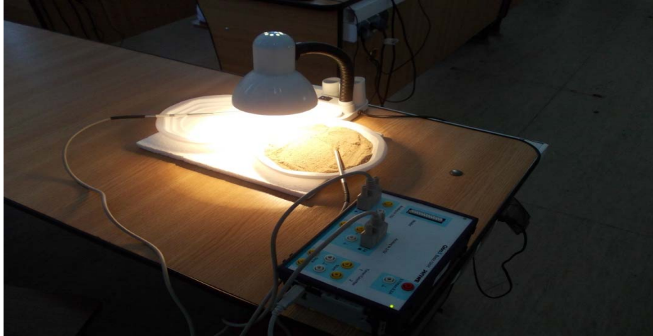
Fig. 1 – Experimental set-up for the experiment Comparison between specific heat of water and sand . The colored versions can be accessed at http://www.infim.ro/rfp/ .
