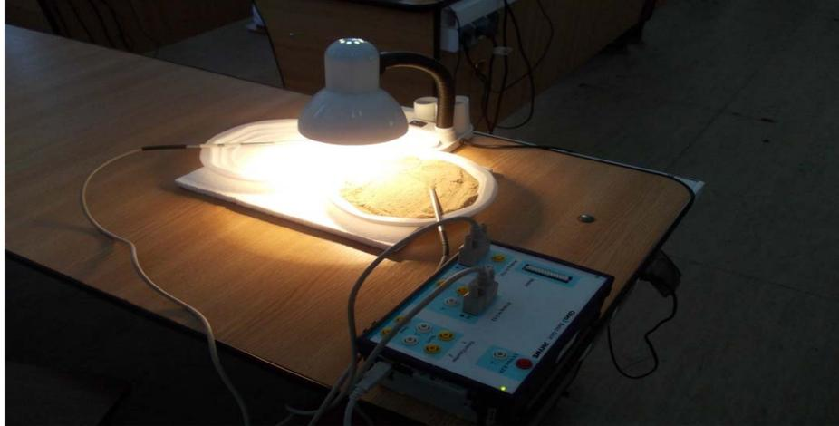
Fig. 1 – Experimental set-up for the experiment *Comparison between specific heat of water and sand*.
