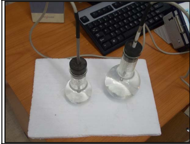
Fig. 5 – Experimental set-up of the „Bergmann’s rule verification experiment” using uninsulated bottom flasks. The colored versions can be accessed at http://www.infim.ro/rp/ .
