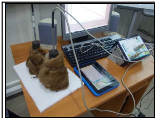
Fig. 8 – The experimental setup to verify the Bergmann's rule using covered round bottoms flasks with fur. The colored versions can be accessed at http://www.infim.ro/rpp/ .
