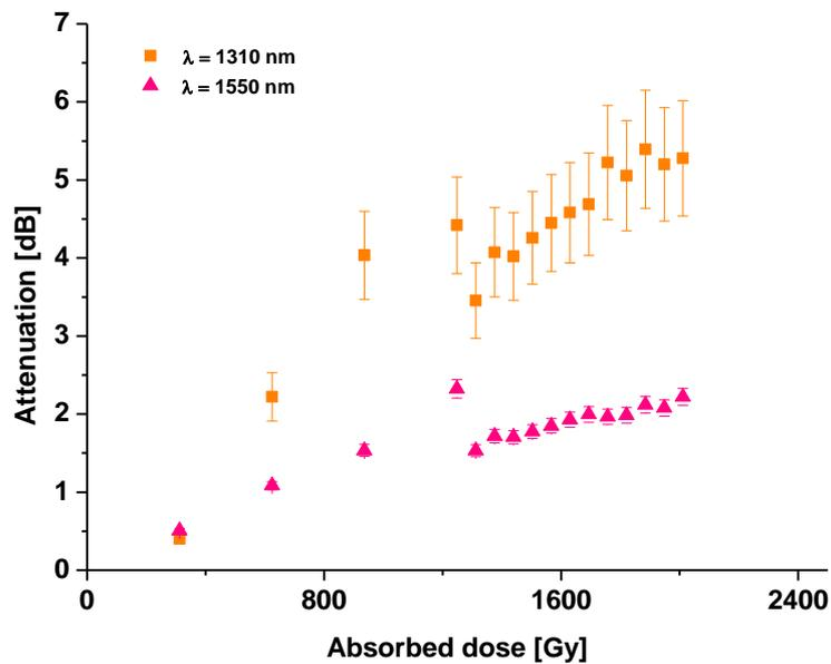
Fig. 3.2.1 – Optical fiber attenuation during exposure to radiation.
