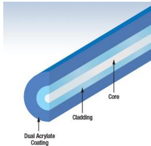
Fig. 2.1 – Structure of ultra-high NA single-mode fiber [4].
