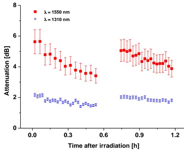
Fig. 3.2.2 – Optical fiber attenuation after an elapsed time.
