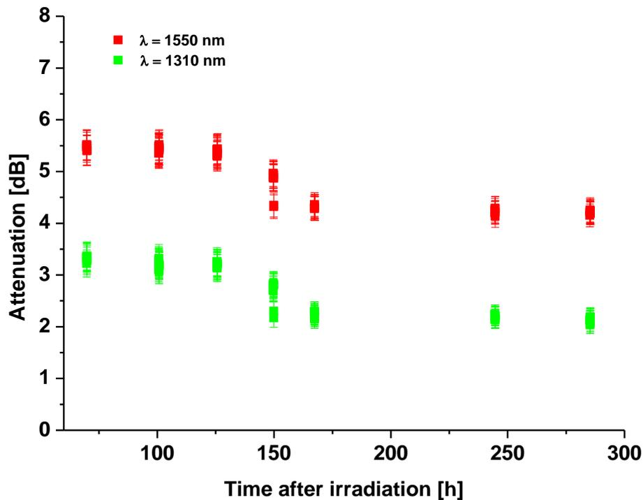
Fig. 3.1.4 – Optical fiber attenuation after an elapsed time of recovery.
