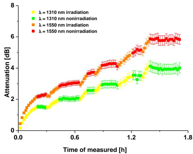
Fig. 3.1.3 – Optical fiber attenuation during exposure to high energy electron beam and after.
