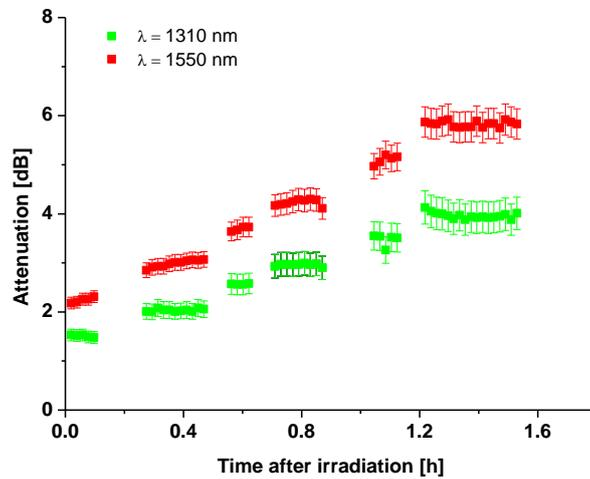
Fig. 3.1.2 – Optical fiber attenuation after an elapsed time in ultra-high NA single-mode fiber.
