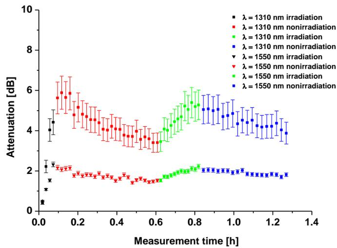
Fig. 3.2.2 – Optical fiber attenuation during exposure to high energy electron beams and after.
