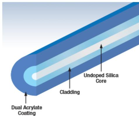
Fig. 2.2 – Structure of photosensitive single mode optical fiber [4].
