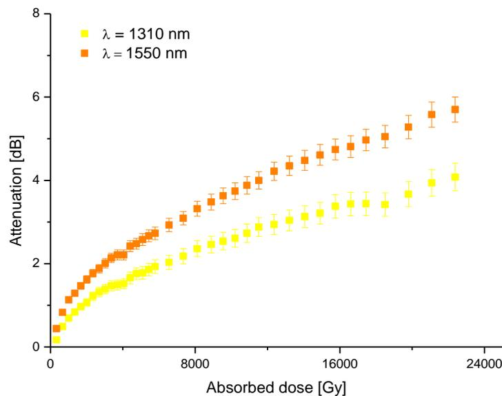
Fig. 3.1.1 – Optical fiber attenuation during exposure to high energy electron beam.
