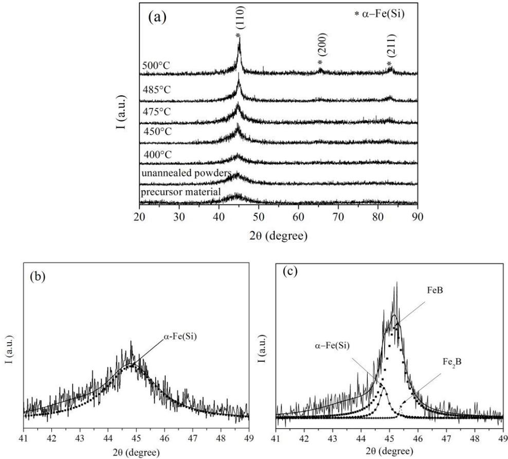
Fig. 3 – XRD patterns for precursor material, unannealed, and annealed powders (a); deconvolution for diffraction peak at  $2\theta = 45^\circ$  for annealed powders at  $475^\circ\text{C}$  (b) and  $500^\circ\text{C}$  (c).
