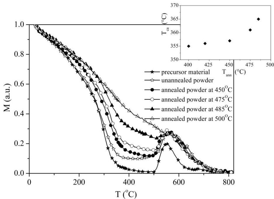
Fig. 2 – Normalized thermomagnetic curves for the precursor material, unannealed powders and isothermally annealed powders and  $T_{ca}$  dependence on  $T_{ann}$  (inset).
