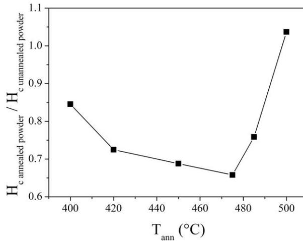
Fig. 4 – The dependence ratio  $H_c \text{ annealed powder} / H_c \text{ unannealed powder}$  on the on annealing temperature.
