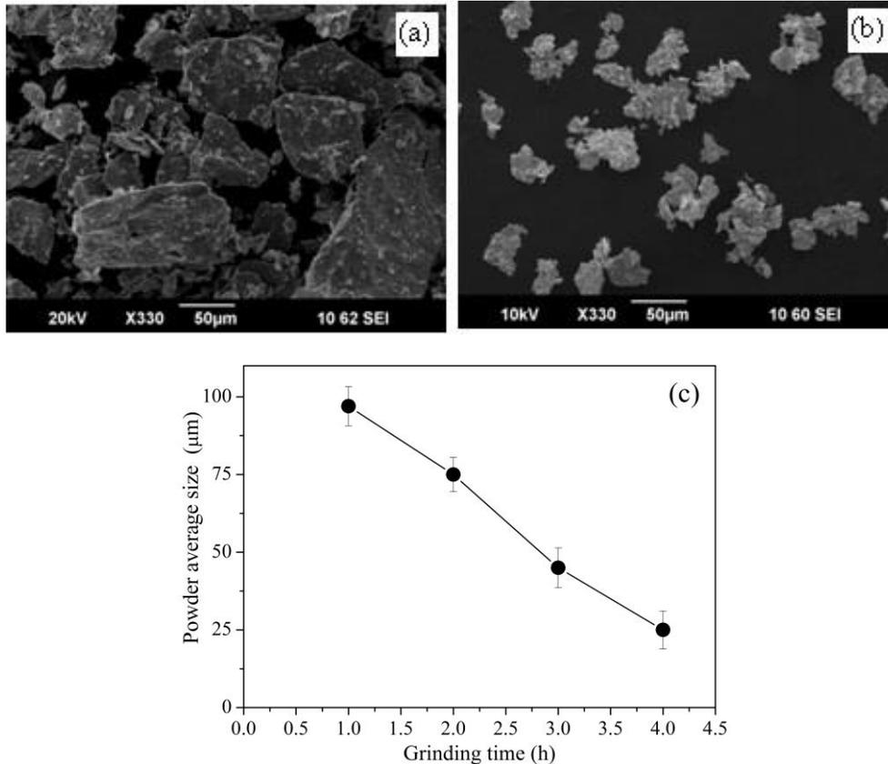
Fig. 1 – SEM images of  $\text{Fe}_{73.5}\text{Cu}_1\text{Nb}_3\text{Si}_{13.5}\text{B}_9$  powders after 1h (a), 4h (b) milling time and the dependence of powder average size on the milling time (c).
