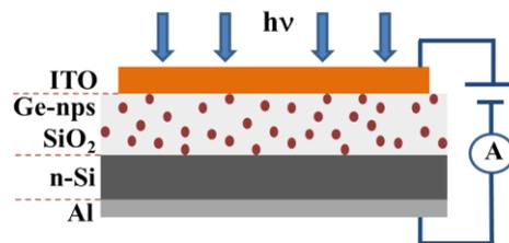
Fig. 1 – Nanostructure configuration and measurement setup schematically.
