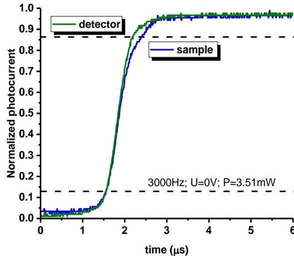
Fig. 4 – Normalized photocurrent response time characteristics. The green line represents the baseline system response ( $\sim 0.6 \mu\text{s}$  response time) obtained under illumination using a  $\lambda = 808.5 \text{ nm}$  laser beam modulated by a mechanical chopper at  $f = 3 \text{ KHz}$  using a commercial InGaAsP photodiode. With blue line is represented the structure photoresponse signal ( $\sim 0.8 \mu\text{s}$  response time).
