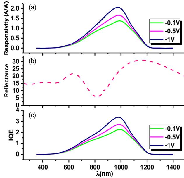
Fig. 3 – a) Spectral responsivity of the investigated structure obtained at various applied reverse bias; b) measured reflectance spectra as a function of excitation wavelength in the range of 350 ÷ 1400 nm; c) internal quantum efficiency (IQE) as a function of wavelength under different reverse bias values.
