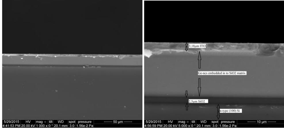
Fig. 2 – Different SEM images of the structure (cross section) which shows the Ge layers for the multilayered structure thickness.
