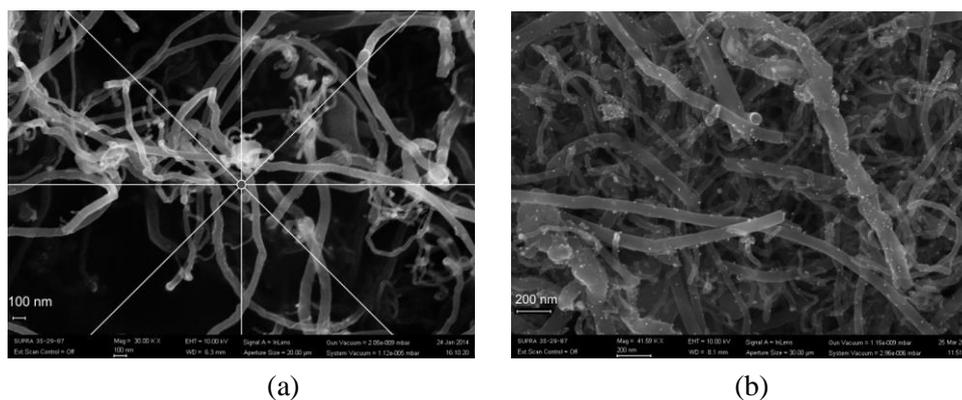
Fig. 1 – SEM photo of (a) pristine MWCNTs and (b) MWCNTs decorated with Au nanoparticles.
