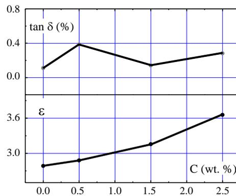
Fig. 5 – Dependence of dielectric parameters on the mass concentration of MWCNTs at 1 kHz and at room temperature.
