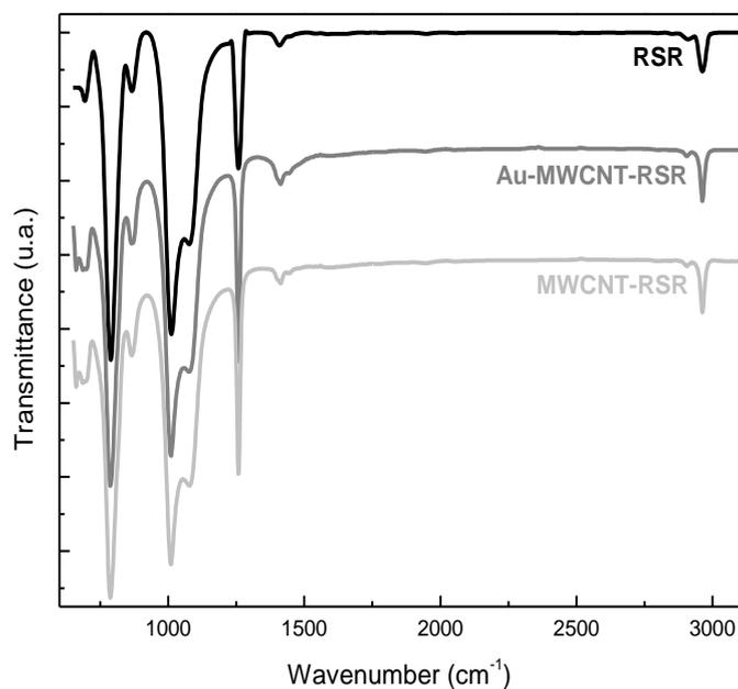
Fig. 2 – ATR-FTIR spectra of RSR and 2.5 wt. % MWCNT-RSR and Au-MWCNT-RSR composites.
