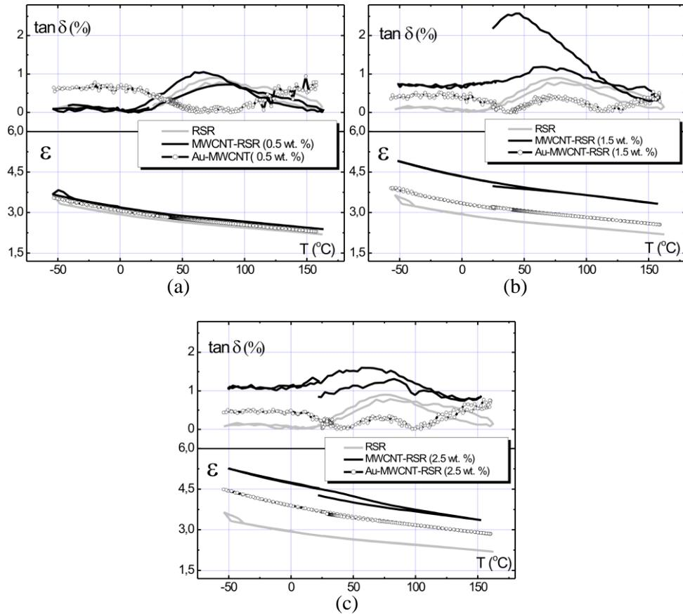
Fig. 6 – Temperature dependence of the permittivity and losses at 1 kHz of RSR, MWCNT-RSR and Au-MWCNT-RSR composites with different Au-MWCNT concentrations: a) 0.5 wt. %; b) 1.5 wt. %; c) 2.5 wt. %.
