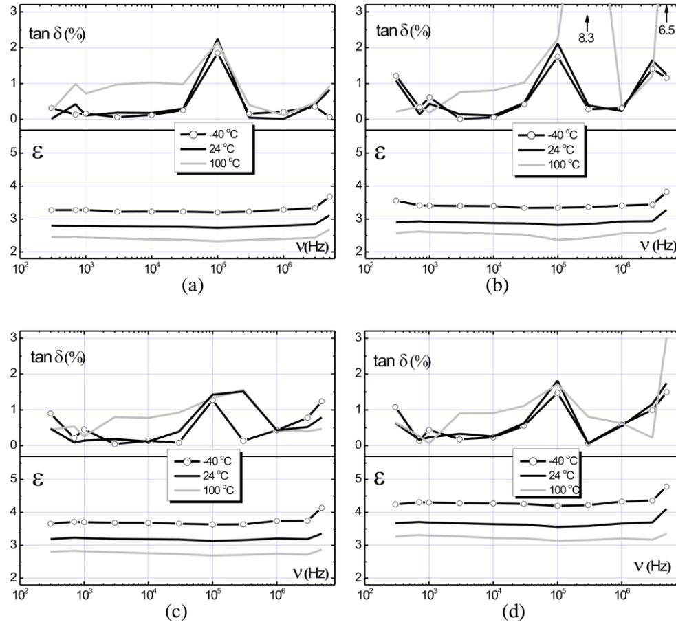
Fig. 7 – Frequency dependence of the permittivity and losses at different temperatures of Au-MWCNT-RSR composites with different Au-MWCNT concentrations: a) 0 wt. %; b) 0.5 wt. %; c) 1.5 wt. %; d) 2.5 wt. %.
