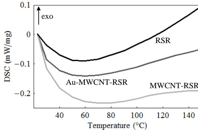
Fig. 3 – Differential Scanning Calorimetry results for the RSR and 2.5 wt. % MWCNT-RSR and Au-MWCNT-RSR composites.
