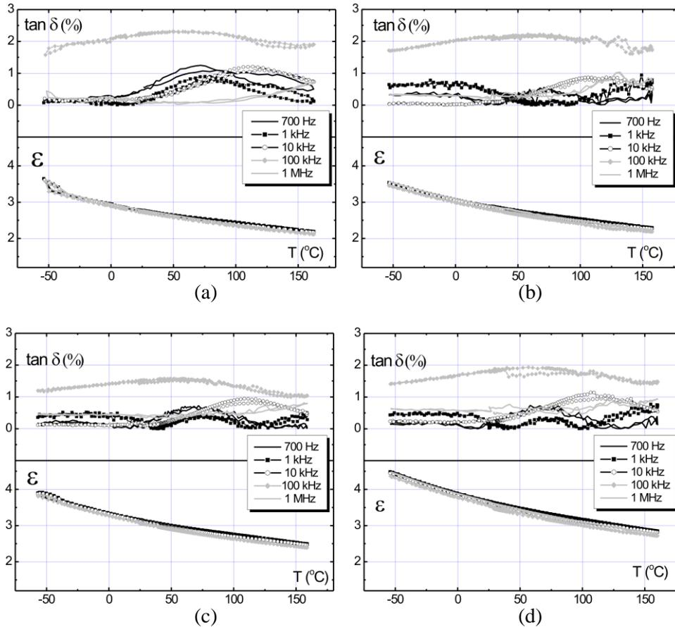
Fig. 4 – Temperature dependence of the permittivity and losses at different frequencies of Au-MWCNT-RSR composites for different Au-MWCNT concentrations: a) 0 wt. %, b) 0.5 wt. %, c) 1.5 wt. %; d) 2.5 wt. %.
