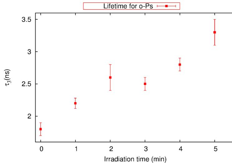
Fig. 2 – o-Ps lifetime for CL normal, irradiated 1,2,3,4,5 minutes.
