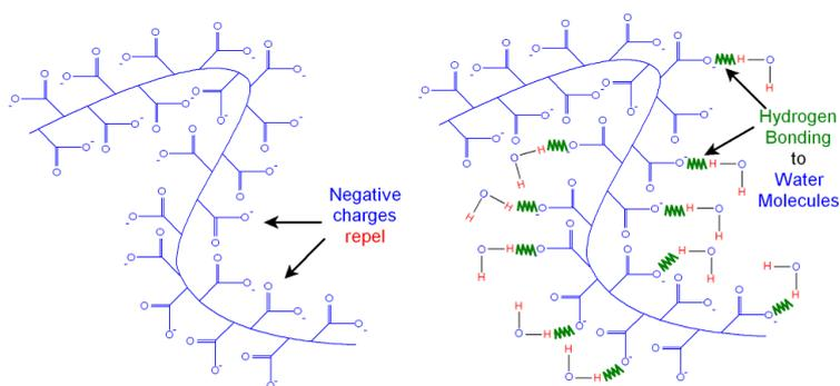
Fig. 1 – Hydrogel schematic view. Hydrogen bonding in hydrogel
